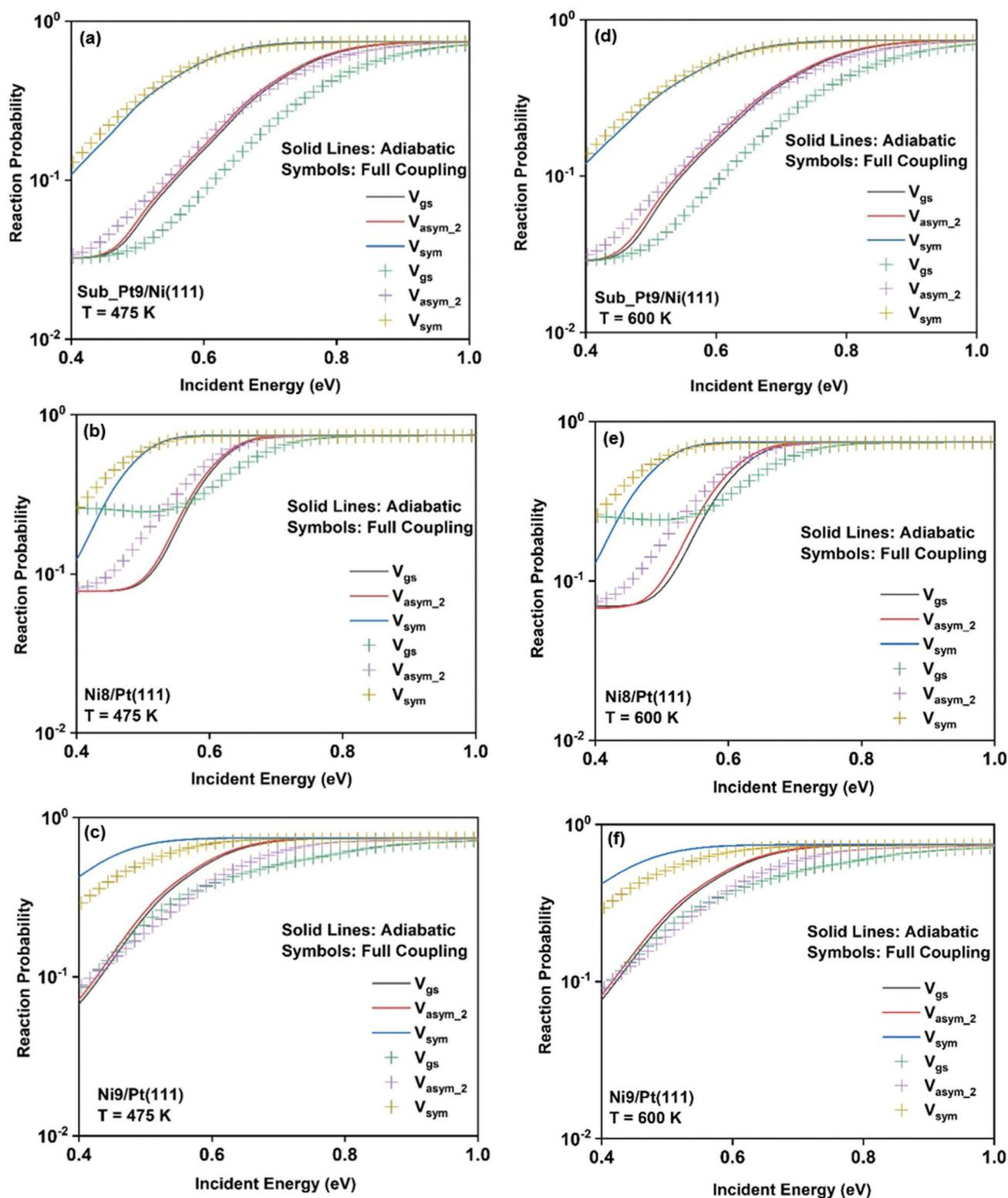
Fig. 7 Adiabatic and full coupling reaction probabilities for  $\text{CH}_4$  in the vibrational ground state, symmetric stretching, and asym\_2 stretching excited state as mentioned in the figure, for the dissociation of  $\text{CH}_4$  at 475 K surface temperature on (a) Sub-Pt9/Ni(111), (b) Ni8/Pt(111), and (c) Ni9/Pt(111) and at 600 K surface temperature on (d) Sub-Pt9/Ni(111), (e) Ni8/Pt(111), and (f) Ni9/Pt(111) alloy surfaces.
