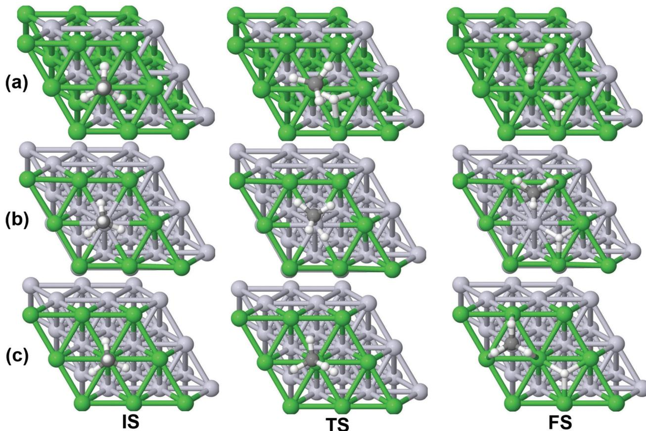
Fig. 1 Optimized structures of the initial state (IS), transition state (TS), and final state (FS) for the dissociation of  $\text{CH}_4$  on (a) Sub-Pt9/Ni(111), (b) Ni8/Pt(111) and (c) Ni9/Pt(111) alloys. The green balls refer to Ni atoms, silver-white balls refer to Pt atoms, small black balls refer to carbon atoms, and small white balls refer to hydrogen atoms.
