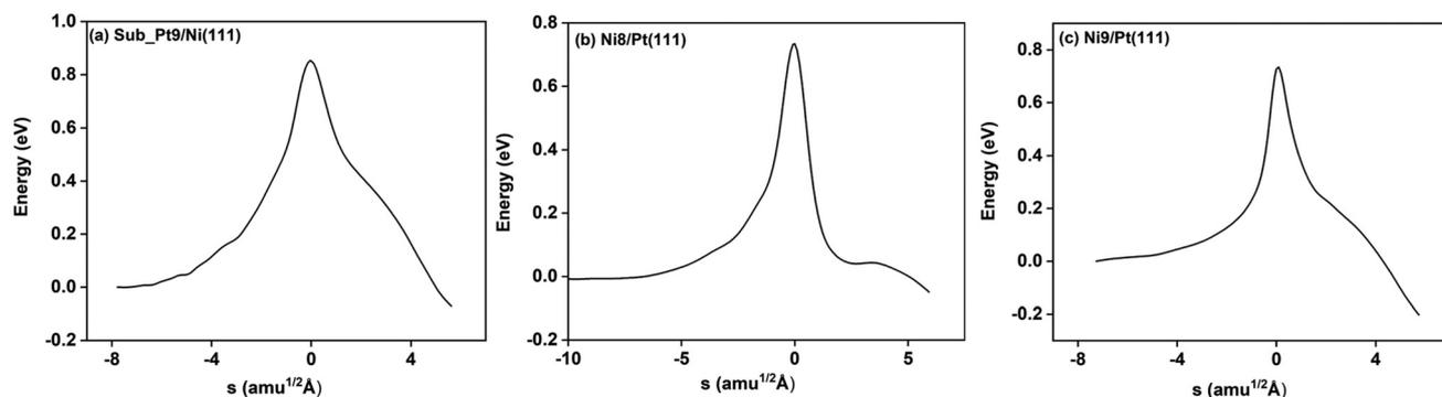
Fig. 2 Reaction path diagram for the methane dissociation on (a) Sub-Pt9/Ni(111), (b) Ni8/Pt(111), and (c) Ni9/Pt(111) surfaces without ZPE corrections. The x axis of the figure is given by  $s$  (reaction path). Negative  $s$  means reactant side,  $s = 0$  indicates transition state and the positive value of  $s$  refers to product side.
