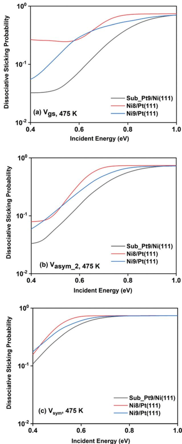
Fig. 9 Comparison of the dissociative sticking probability of (a) the vibrational ground state and of normal modes excited by one-quantum in (b) symmetric and (c) asym\_2 stretching modes for CH<sub>4</sub> dissociation on the three studied alloy surfaces calculated at 475 K to underline how the alloying changes the reactivity for the methane dissociation process.
