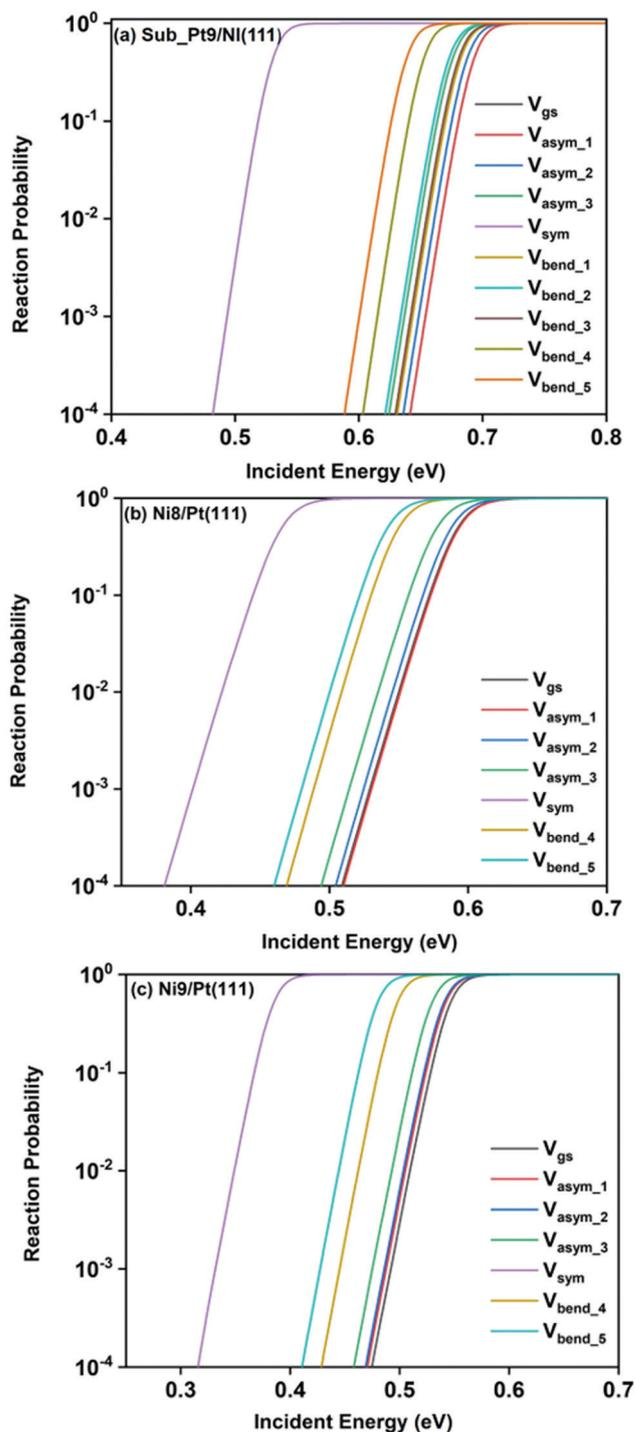
Fig. 5 Reaction probabilities within the vibrationally adiabatic limit under the static surface approximation as a function of incident energies for CH<sub>4</sub> in the vibrational ground state and several other initial vibrationally excited state as mentioned in the figure, for CH<sub>4</sub> dissociation on (a) Sub-Pt9/Ni(111), (b) Ni8/Pt(111), and (c) Ni9/Pt(111) alloy surfaces.
