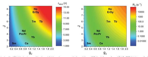
Fig. 4 Typical radii of  $^{1}$ H blind spheres of lanthanoid(III) ions (paramagnetic linewidths  $\geq$ 100 Hz, left panel), and  $^{1}$ H  $R_{2}$  PRE (right panel), due to Curie relaxation, for a proton at 10 Å from the lanthanoid ion, at 900 MHz. The electron relaxation times  $\tau_e$  are set to 1 ps and  $\tau_r$  to 10 ns. Gadolinium(III), with  $\tau_e$ several orders of magnitude larger, is shown in Fig. 3.
