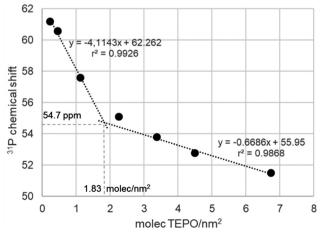
Fig. 3 Variation of <sup>31</sup>P chemical shift (ppm) of adsorbed TEPO at different surface coverages on Aerosil 200 calcined at 500 °C.
