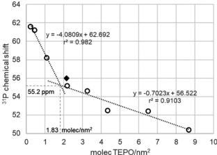
Fig. 5 Variation of <sup>31</sup>P chemical shift (ppm) of adsorbed TEPO at different surface coverages on Aerosil 200 calcined at 200 °C. Diamond: result described for silica gel in ref. 5
