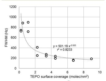
Fig. 6 Dependence of the linewidth of TEPO <sup>31</sup>P signal with the surface coverage in the case of Aerosil 200.
