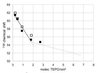
**Fig. 7** Variation of  $^{31}$ P chemical shift (ppm) of adsorbed TEPO at different surface coverages on MCM-41 calcined at 500  $^{\circ}$ C (filled squares and dotted line) and 200  $^{\circ}$ C (open squares). The tendency lines for TEPO adsorbed on Aerosil calcined at 500  $^{\circ}$ C are included in grey for the sake of comparison.
