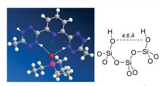
Fig. 4 Measurement of the N-N distance in the H<sub>4</sub>btzp<sup>Me</sup>·OPEt<sub>3</sub> complex<sup>29</sup> and comparison with the O-O distance between two neighbour isolated silanols in a model<sup>30</sup> of amorphous silica surface.
