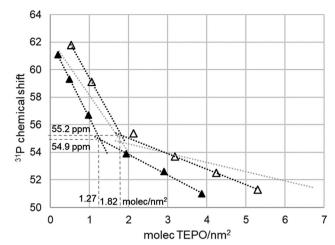
Fig. 8 Variation of  $^{31}$ P chemical shift (ppm) of adsorbed TEPO at different surface coverages on Silia P60 calcined at 500 °C (filled symbols) and 200 °C (open symbols). The tendency lines for TEPO adsorbed on Aerosil calcined at 500 °C are included in grey for the sake of comparison.
