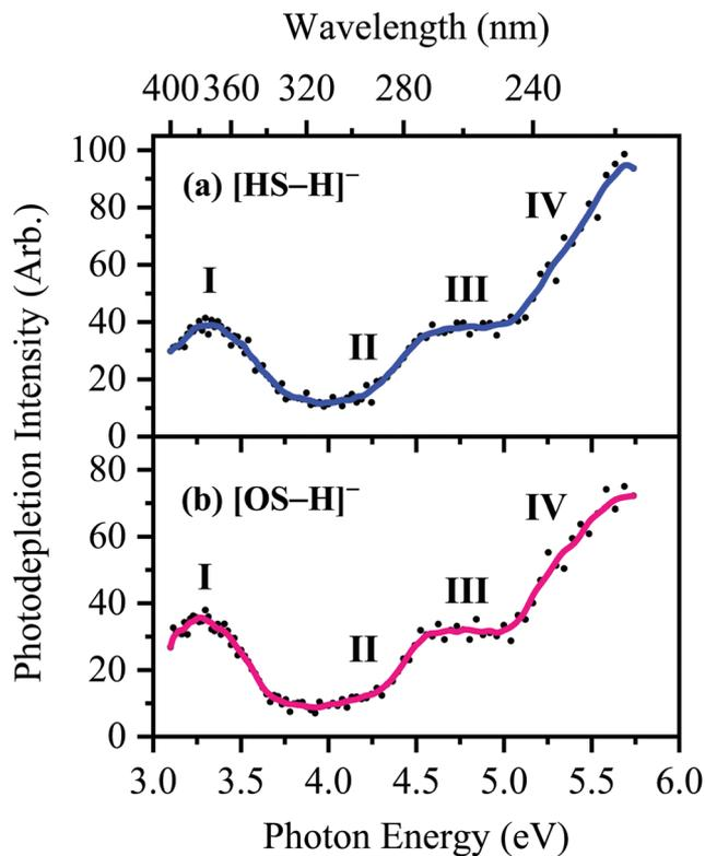
Fig. 2 Gas-phase UV absorption (photodepletion) spectra of (a)  $[\text{HS} - \text{H}]^-$  and (b)  $[\text{OS} - \text{H}]^-$ , respectively. The solid line is a five-point adjacent average of the data points.
