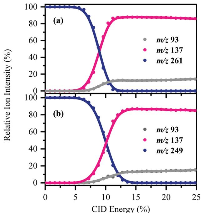
Fig. 3 CID fragmentation curves of (a)  $[\text{HS} - \text{H}]^-$  and (b)  $[\text{OS} - \text{H}]^-$  between 0–25% CID energy. Onset plots for production of the associated fragment ions ( $m/z$  93 and 137) are also shown. The curved lines are a three-point adjacent average of the data points.
