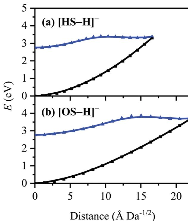
Fig. 6 Energies of the  $S_0$  (black) and  $S_1$  (blue) states between the  $S_0$  minimum-energy geometries/Franck-Condon points and the  $S_0 \leftarrow S_1$  MECP of (a)  $[\text{HS} - \text{H}]^-$  and (b)  $[\text{OS} - \text{H}]^-$ . Points were generated via linear interpolation of internal coordinates (LIIC). Energies were evaluated at the [RI-MP2/ADC(2)]/aug-cc-pVDZ level.
