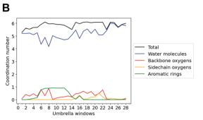
Fig. 5 Coordination number of Na<sup>+</sup> during umbrella sampling simulation in ASIC1. (A) Coordination number of the permeating Na<sup>+</sup> for the last 28 windows in 4NTW. (B) Coordination number of the permeating Na<sup>+</sup> in 6VTK
