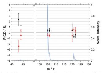
Fig. 4 PICD values, measured in coincidence, phenylethylamine (black) and S-(-)-1-phenylethylamine (red) and the mass spectrum (blue) for the multiphoton excitation at 394.4 nm. The plotted PICD values are symmetrized. The raw and symmetrized PICD values are listed in Table 2.
