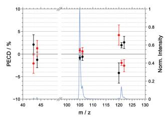
Fig. 6 Symmetrized PECD values, measured in coincidence, for R-(+)-1phenylethylamine (black) and S-(-)-1-phenylethylamine (red) and the mass spectrum (blue) for the multiphoton excitation at 394.4 nm. The raw data are listed in Table 3.
