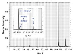
Fig. 3 Measured mass spectrum of 1-phenylethylamine using a static electric field of 1000 V cm<sup>-1</sup> in the ionization region (non-coincidence conditions). Data from R-(+)-1-phenylethylamine with the left circular polarized light are shown. Measurements on the other enantiomer and/ or other circular polarization yielded the same fragmentation pattern, with minor differences (1-2%) in the absolute yield of the different ion masses. The inset is a zoom-in on the mass region at m/z > 100.
