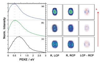
Fig. 7 Photoelectron kinetic energy (PEKE) distributions, the photoelectron images for measurement with the LCP and RCP and the difference image for the dominant ions of R-(+)-1-phenylethylamine measured in coincidence after multiphoton ionization at 394.4 nm for (a) [M-NH<sub>2</sub>]<sup>+</sup> (m/z = 105), (b) composite (m/z = 106) and (c) parent ion (m/z = 121). The laser propagation direction is indicated by the red arrow.
