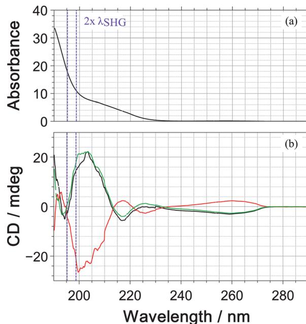
Fig. 5 Absorption spectrum (a) and CD spectrum (ellipticity in units of mdeg) (b) of 1-phenylethylamine (1-PEA) in acetonitrile measured using a Jasco J-815 CD-spectrometer. The spectra of *R*-(+)-1-PEA (black), *S*-(-)-1-PEA (red) and the symmetrized trace (green) are shown. The purple lines indicate the 2-photon absorption bandwidth of our laser pulses.
