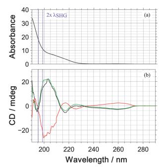
Fig. 5 Absorption spectrum (a) and CD spectrum (elipticity in units of mdeg) (b) of 1-phenylethylamine (1-PEA) in acetronitrile measured using a Jasco J-815 CD-spectrometer. The spectra of R-(+)-1-PEA (black), S-(-)-1-PEA (red) and the symmetrized trace (green) are shown. The purple lines indicate the 2-photon absorption bandwidth of our laser pulses.
