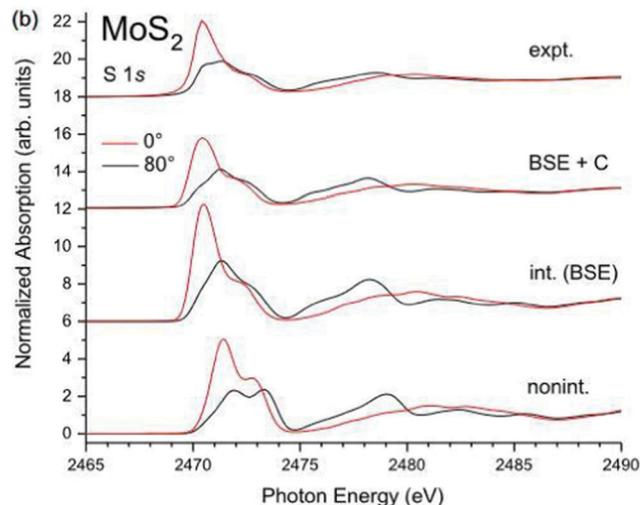
Fig. 11 K-Edge XAS of MoS<sub>2</sub> calculated within the non-interacting approximation (bottom), BSE (second curves), and BSE + cumulant (third curves), compared to experiment (top). The angle of polarization is shown by the colors. Reprinted figure with permission from [J. C. Woicik, C. Weiland, A. K. Rumaiz, M. T. Brumbach, J. M. Ablett, E. L. Shirley, J. J. Kas and J. J. Rehr, *Phys. Rev. B*, 2020, **101**, 245105], Copyright (2022) by the American Physical Society.
