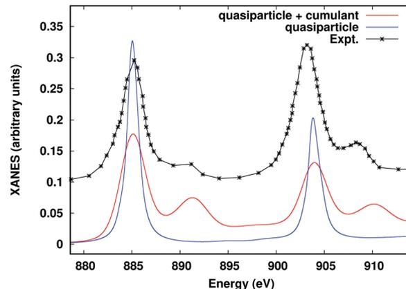
Fig. 14 Ce M-edge XANES of CeO<sub>2</sub> including the many-body convolution with the cumulant spectral function compared to the quasiparticle spectrum and experiment.<sup>88</sup>
