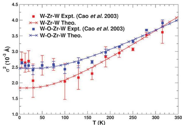
Fig. 5 Calculated MSRD of various paths in  $\text{ZrW}_2\text{O}_8$  compared with experimental results. Reprinted figure with permission from [F. D. Vila, J. W. Spencer, J. J. Kas, J. J. Rehr and F. Bridges, *Front. Chem.*, 2018, **6**, 1].
