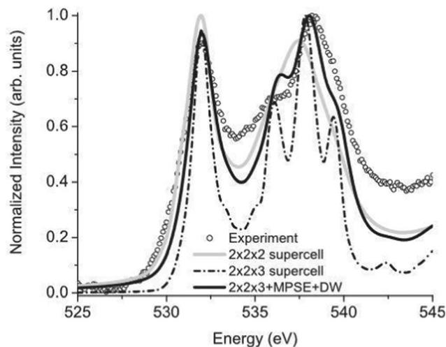
Fig. 3 Many-pole self-energy (MPSE) applied to calculations of the O K-edge spectrum of SnO<sub>2</sub>. Reprinted figure with permission from [M. S. Moreno, J. J. Kas, C. Ma, F. Wang, J. J. Rehr and M. Malac, *Phys. Rev. B*, 2017, **95**, 245206], Copyright (2022) by the American Physical Society.
