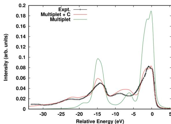
Fig. 12 Fe 2p XPS of  $\alpha$ -Fe<sub>2</sub>O<sub>3</sub> calculated within the multiple + C approach (red) compared to the multiplet-only spectrum (green), and experimental results (black crosses). Reprinted figure with permission from [J. J. Kas, J. J. Rehr and T. P. Devereaux, *Ab initio* multiplet plus cumulant approach for correlation effects in X-ray photoelectron spectroscopy, 2021, <https://arxiv.org/abs/2107.10409>].
