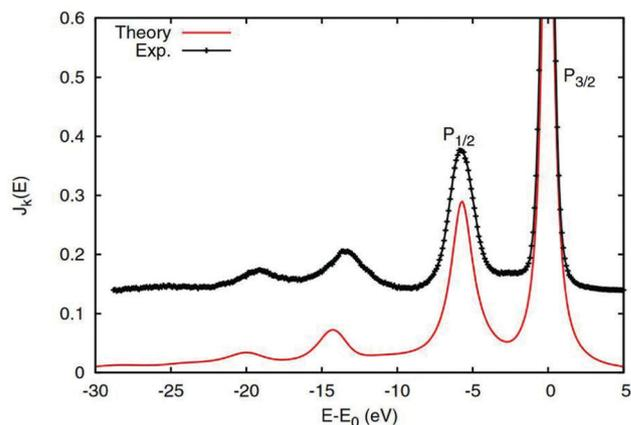
Fig. 9 2p core-level XPS of rutile TiO<sub>2</sub> calculated with the real-time cumulant approach (red solid) compared to experimental results (black). The main quasiparticle peaks are labeled  $P_{1/2}$  and  $P_{3/2}$ , while the charge transfer satellites appear at ~14 eV lower energy. Reprinted figure with permission from [J. J. Kas, F. D. Vila, J. J. Rehr and S. A. Chambers, *Phys. Rev. B*, 2015, **91**, 121112], Copyright (2022) by the American Physical Society.
