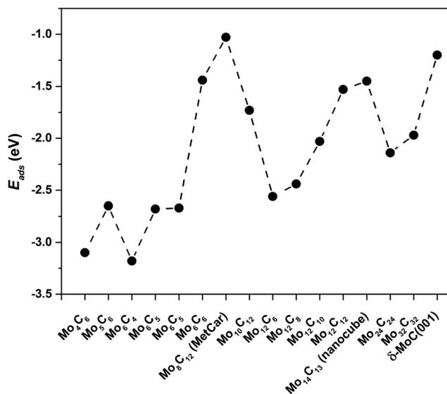
Fig. 8 CO<sub>2</sub> adsorption energy,  $E_{\text{ads}}$ , for the most stable CO<sub>2</sub> bonding mode on the different nanoparticles.
