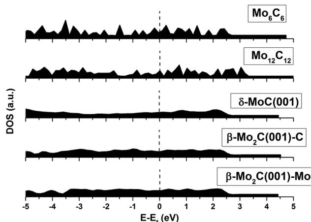
Fig. 4 Density of states (DOS) for the bare carbide nanoparticles and surfaces. The β-Mo<sub>2</sub>C(001) surface has C- and Mo-terminations, hence, both surfaces are included. Mo<sub>6</sub>C<sub>6</sub> and Mo<sub>12</sub>C<sub>12</sub> were taken as representative nanoparticles.
