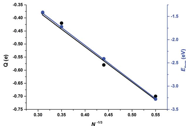
**Fig. 6** Bader charge ( $Q$ ) in adsorbed  $\text{CO}_2$  (left) and nanoparticle cohesion energy per MoC unit ( $E_{\text{form}}$ , right) versus the particle size defined as  $N^{-1/3}$ ,  $N$  being the number of MoC units. Note that with this definition the bulk value is zero. Linear regressions are included for black and blue lines, with  $R^2$  values of 0.986 and 0.999, respectively.
