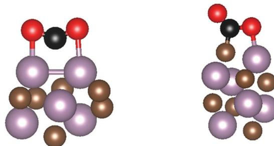
Fig. 3 Atomistic views of the  $\eta^3\text{-CO}_2\text{-}\mu^2\text{-C}_B\text{O}_M\text{O}_M$  (left) and  $\eta^2\text{-CO}_2\text{-}\mu^2\text{-C}_C\text{O}_M$  (right) adsorption modes seen on two different carbide nanoparticles. C, Mo and O atoms are shown as brown, magenta, and red spheres, respectively. The C atom in  $\text{CO}_2$  is shown as a black sphere.
