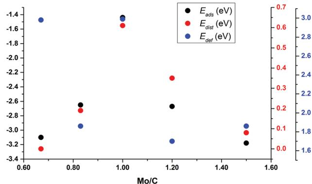
**Fig. 7** For non-stoichiometric nanoparticles derived from Mo<sub>6</sub>C<sub>6</sub>, Relationship between the Mo/C ratio and CO<sub>2</sub> adsorption energy,  $E_{\text{ads}}$  (left axis, in black) or the nanoparticle distortion energy,  $E_{\text{dist}}$  (right axis, in red), or CO<sub>2</sub> deformation energy,  $E_{\text{def}}$  (right, in blue).
