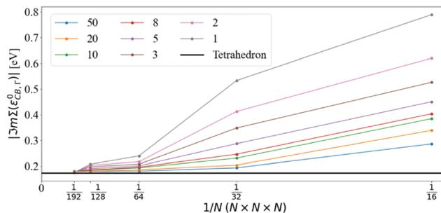
**Fig. 3** Convergence of  $\Im m\Sigma_{c\Gamma}(\epsilon_{c\Gamma}^0)$  using the DM approach with  $N$  for different values of  $\eta = 50, 20, 10, 8, 5, 3, 2$ , and  $1$  meV (indicated in the legend) at 300 K. The black line denotes the reference value obtained with the tetrahedron method and  $N = 160$ .
