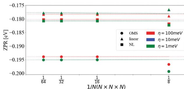
Fig. 1 ZPR for the CBM as a function of the number of divisions in the  $\mathbf{q}$ -mesh and different values of  $\eta$ . The data was fitted with a linear model and extrapolated for  $1/N \rightarrow 0$ . Calculations were done with the OMS approach eqn (16) (circles), the linear approximation eqn (14) (triangles) and the non-linear approach eqn (13) (squares). The values obtained with  $\eta = 10$  meV and  $\eta = 1$  meV are indistinguishable on the scale of the graph.
