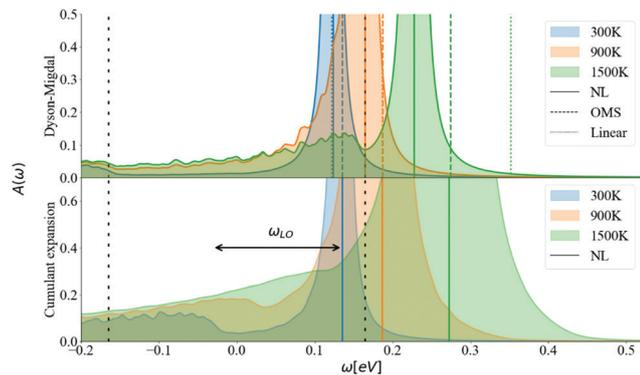
**Fig. 11** Spectral function calculated at the VBM at 300, 900, 1500 (K) using DM and CE methods. The vertical colored lines show the QP energy calculated using non-linear (NL), on-the-mass-shell (OMS) and linear approaches. The vertical dashed black lines correspond to  $\pm\omega_{\text{LO}}$ .  $\eta$  is set to 5 meV and  $N = 128$ .
