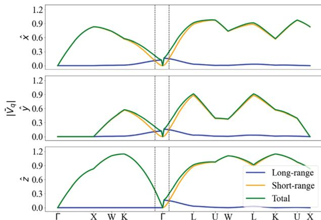
**Fig. 14** Unit-cell average and absolute value of the total DFPT scattering potential (green) compared with the long-range part (blue) and the short-range contribution (orange). The three subplots corresponds to the e-ph potential generated by the displacement of a C atom along one of the three reduced directions  $\hat{x}$ ,  $\hat{y}$ ,  $\hat{z}$ . Both atoms present the same  $|\bar{V}_{\mathbf{q}}|$ .
