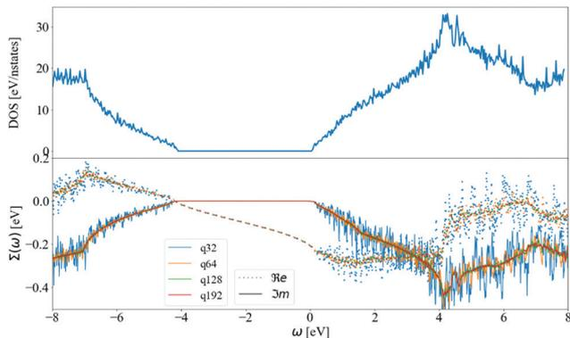
Fig. 5 The (a) density of states and (b) self-energy at CBM and 300 K calculated using DM and  $\eta = 5$  meV for  $N = 32, 64, 128$  and 192 at CBM. The DOS is plotted as a reference, showing its similarity with the imaginary part of the self-energy. Self-energy becomes smooth and converged at  $N = 128$  in green (difficult to visualize) with very small oscillations around the  $N = 192$  data in red (easy to visualize).
