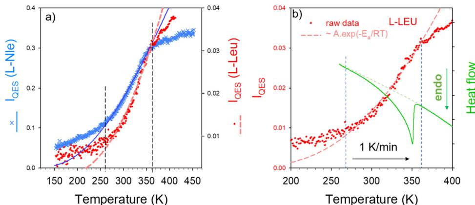
Fig. 4 Temperature dependence of the quasielastic intensity ( $I_{\text{QES}}$ ); (a) comparison of  $I_{\text{QES}}(T)$  in L-LEU and L-Nle, (b) comparison of  $I_{\text{QES}}(T)$  with the heat flow trace in L-LEU.
