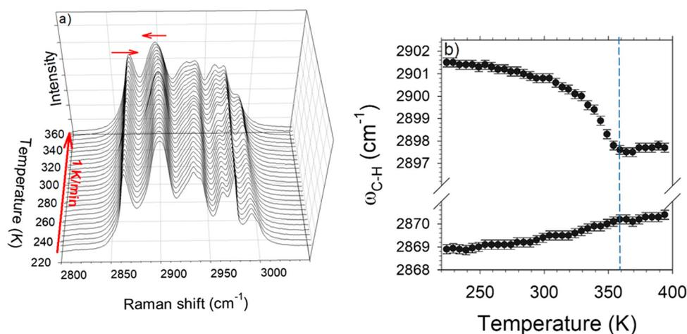
Fig. 5 Temperature dependence of C–H stretching vibrations. (a) Plot of spectra collected during a heating ramp from 220 K at 1 K min<sup>-1</sup>. The horizontal arrows show the opposite temperature dependence of the lowest frequency bands in the C–H stretching region. (b) Temperature dependence of the frequencies of the C–H stretching bands schematically displayed by the arrows in the plot of spectra.
