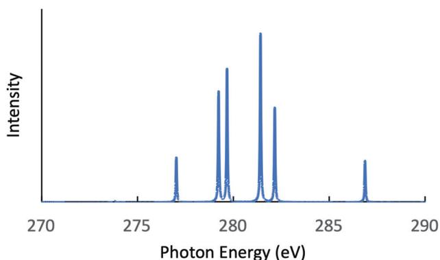
Fig. 2 Calculated RIXS spectrum for CH<sub>3</sub>OH.
