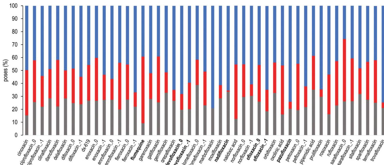
**Fig. 5** Sub-region distribution of the docking poses (%): gray bars refer to the interface, red to the cave, and blue to the groove. FQs are in ascending order according to the molecular weight. FQs containing the piperazine group are reported in two net charges (*i.e.*, 0 and  $-1$ ). LFX and related compounds (Fig. 1) are highlighted in boldface.
