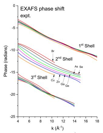
Fig. 11 Experimental phase functions  $\psi_{\rm expt}(k) = 2\delta_1^{'}(k) + \phi(k)$  corresponding to single scattering from the first, second, and third shells. Each set of phase shifts has been displaced by  $2\pi$  radians for clarity (see text).
