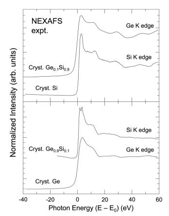
Fig. 2 Sensitivity of XAFS to backscattering environment. Top: Si K edge of crystalline Si and Ge K edge of a dilute Ge in Si crystalline  $Ge_{0.1}Si_{0.9}$  alloy. Bottom: Ge K edge of crystalline Ge and Si K edge of a dilute Si in Ge crystalline  $Ge_{0.9}Si_{0.1}$  alloy. The splitting of the white line (or "rabbit ears") observed at the Si K edge is a density of states effect (see text). (After Woicik and Pianetta.  $^{10}$ )
