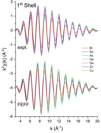
**Fig. 8** First-shell, single-scattering contributions to the EXAFS shown in Fig. 3 compared to their FEFF simulations. The FEFF simulations include  $\sigma^2$ , but not  $S_0^2$  or  $E_0$  corrections (see text).
