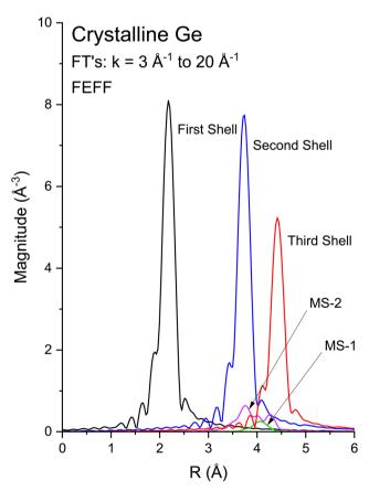
Fig. 5 FEFF path analysis of the diamond crystal structure for crystalline Ge. Note that the first three single-scattering paths are well resolved in R, and the two multiple scattering paths make only a small contribution to the total scattering for the k range  $k = 3 \text{ Å}^{-1}$  to 20 Å<sup>-1</sup> (see text).
