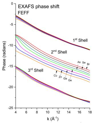
Fig. 12 Theoretical FEFF phase functions  $\psi_{\text{theory}}(k) = 2\delta_1'(k) + \phi(k)$ corresponding to single scattering from the first, second, and third shells. Each set of phase shifts has been displaced by  $2\pi$  radians for clarity (see text).
