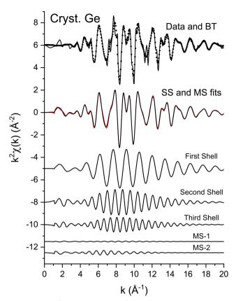
Fig. 14 Upper:  $k^2$ -Weighted EXAFS,  $k^2\chi(k)$ , for crystalline Ge (solid line) plotted with its Fourier-filtered first three-shell contribution (dots). Immediately below are single-scattering (black) and multiple-scattering (red) fits to the filtered data. Lower: Individual scattering contributions: first-, second-, and third-shell single-scattering paths and the multiplescattering paths 1 and 2 (see text).
