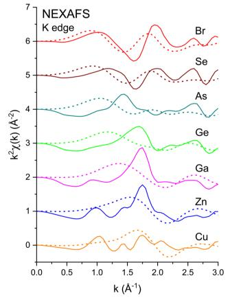
Fig. 6 The XANES or low-k region of the EXAFS shown in Fig. 3 compared to its FEFF simulation for  $R_{\text{max}}$  = 6 Å: Solid line: Experiment. Dashed line: FEFF. Note the high-frequency contributions to the data are not reproduced by the FEFF simulations (see text)
