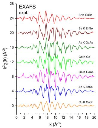
Fig. 3  $k^2$ -Weighted EXAFS,  $k^2\chi(k)$ , for crystalline CuBr, ZnSe, GaAs, and Ge recorded at the Cu, Zn, Ga, Ge, As, Se, and Br K edges. All data were recorded at  $LN_2$  temperature. The zero of the k axis was defined as the maximum of the first derivative of the edge jump (see text).
