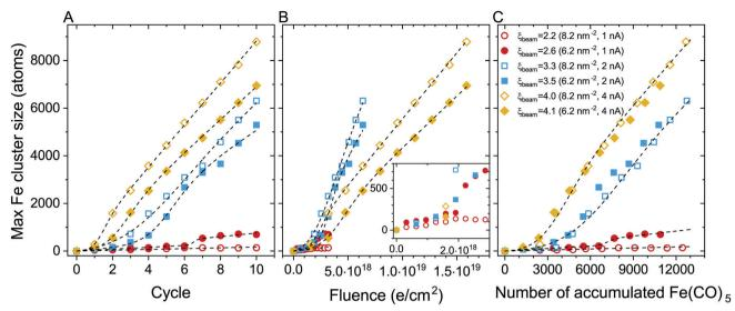
Fig. 4 The maximal number of iron atoms in the largest cluster,  $N_{\text{max}}$ , as a function of FEBID cycle (panel A), electron fluence (panel B) and the number of adsorbed  $Fe(CO)_5$  precursors (panel C) for different irradiation-replenishment conditions considered in this study. Each  $N_{max}$  value has been evaluated at the end of each consecutive FEBID cycle. The dashed lines are plotted to guide the eye. The inset in panel B shows a zoomed-in region of low electron
