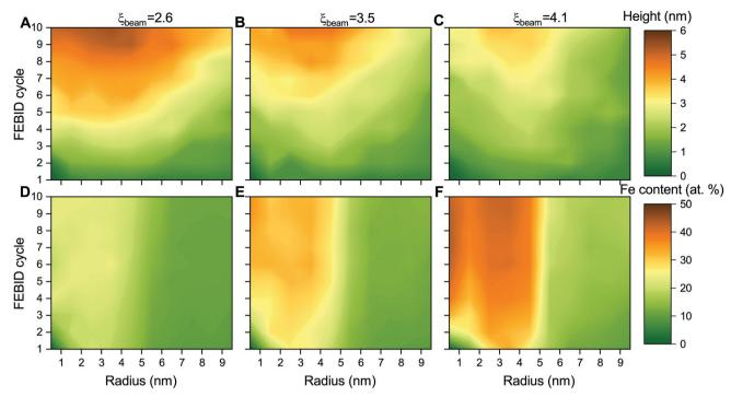
Fig. 5 Radial distribution of the height (panels A–C) and the atomic Fe content (panels D–F) of the grown iron-containing structures as functions of the number of simulated FEBID cycles for electron currents of 1 nA ( $\xi_{beam} \approx 2.6$ ), 2 nA ( $\xi_{beam} \approx 3.5$ ) and 4 nA ( $\xi_{beam} \approx 4.1$ ).
