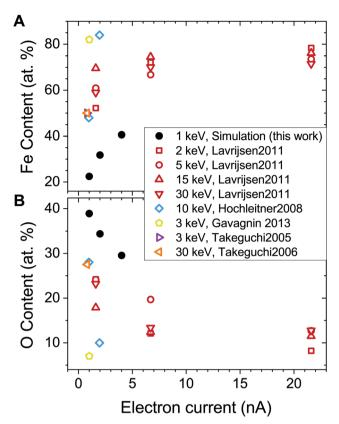
Fig. 7 Fe (panel A) and O (panel B) content in the deposited structures as a function of electron current. Solid black dots correspond to the values obtained in the present study. Open symbols show experimental data from ref. 27, 28, 32, 56 and 57. Note that the FEBID experiments by Lavrijsen et al.<sup>27</sup> were carried out for Fe<sub>2</sub>(CO)<sub>9</sub> precursors.
