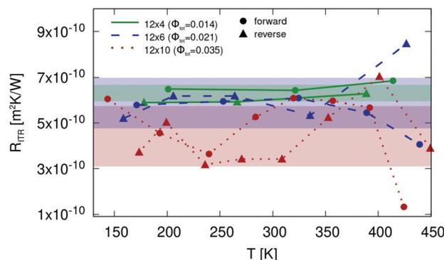
Fig. 8 Interface thermal resistance  $R_{\text{ITR}}$  as a function of temperature in forward (circles) and reverse (triangles) bias, calculated for samples  $12 \times 4$  (green solid lines),  $12 \times 6$  (blue dashed lines) and  $12 \times 10$  (red dotted lines). Shaded areas represent the corresponding standard deviation  $\Delta R_{\text{ITR}}$ .
