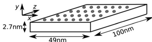
Fig. 1 Sketch of the Si membrane samples that have been analyzed in this work. Heat flow has been simulated in *z*-direction.
