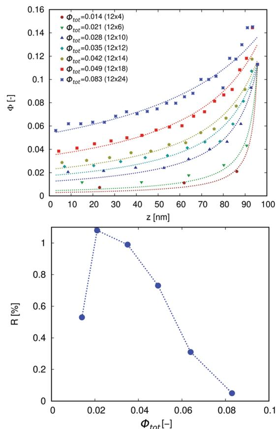
Fig. 6 Porosity (top) as a function of  $z$  and thermal rectification (bottom) as a function of the total porosity  $\phi_{\text{tot}}$  for ordered pore distribution in samples with fixed interface porosity of  $\phi_{\perp} = 0.22$ .
