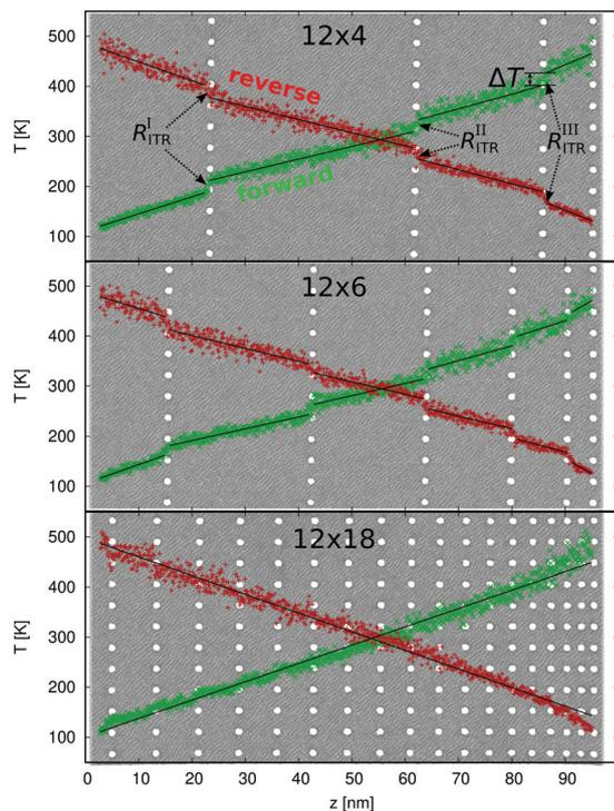
Fig. 7 Temperature profile in forward (x) and reverse (+) bias for samples with ordered pore distribution and an overall porosity  $\Phi_{\text{tot}}$  of 0.014 ( $12 \times 4$ , top), 0.021 ( $12 \times 6$ , center) and 0.064 ( $12 \times 18$ , bottom). The background of each panel shows the top view on the corresponding sample.
