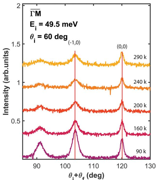
Fig. 3 Angular distribution of He scattered by PdTe<sub>2</sub> as a function of surface temperature, taken at an incident energy of 49.5 meV, along  $\overline{\Gamma M}$ .
