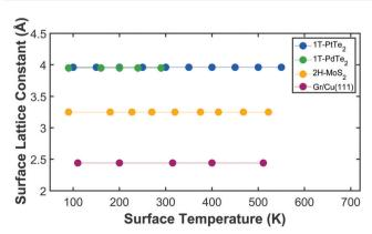
Fig. 4 Comparison of the lattice constant as a function of surface temperature derived from HAS data in four different 2D materials
