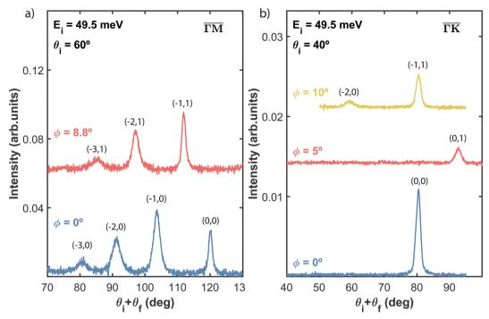
Fig. 2 Angular distributions of He scattered from the PdTe<sub>2</sub> surface kept at 90 K, in-plane (blue curves) and out-of-plane (red and yellow curves), taken along the two main symmetry directions  $\overline{\Gamma} \overline{M}$  and  $\overline{\Gamma} \overline{K}$ . The energy of the incident He beam is  $E_i = 49.5$  meV.
