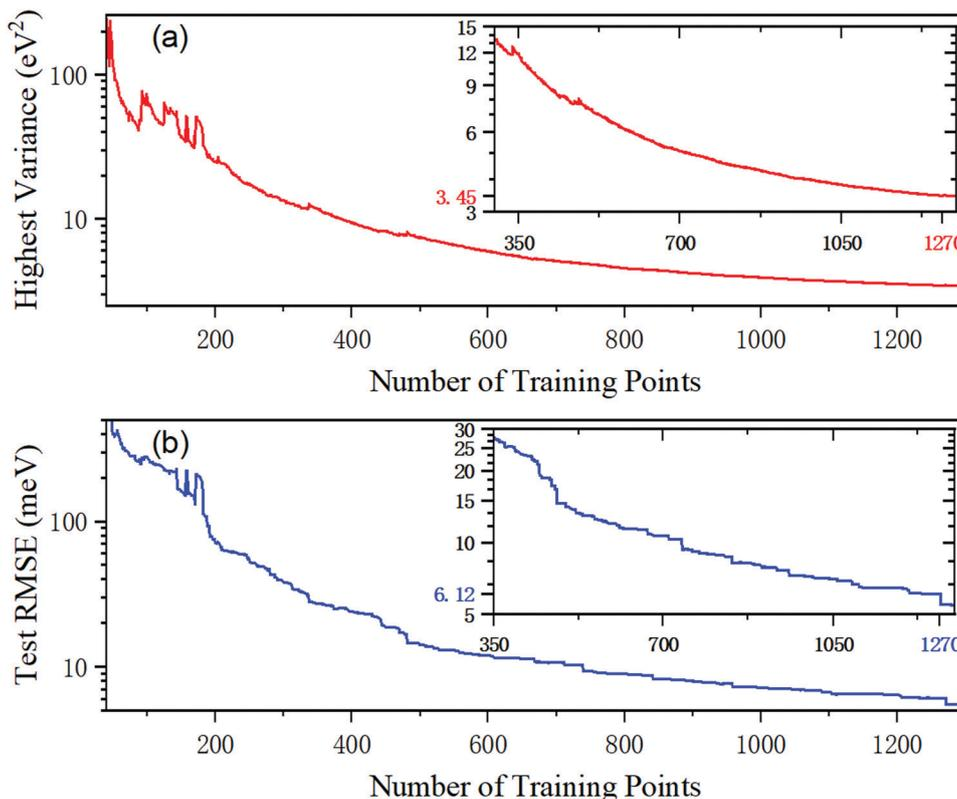
Fig. 2 The highest predictive variance and the RMSE of the test database as a function of the number of training points in the GPR training for the BeH<sub>2</sub><sup>+</sup> system.
