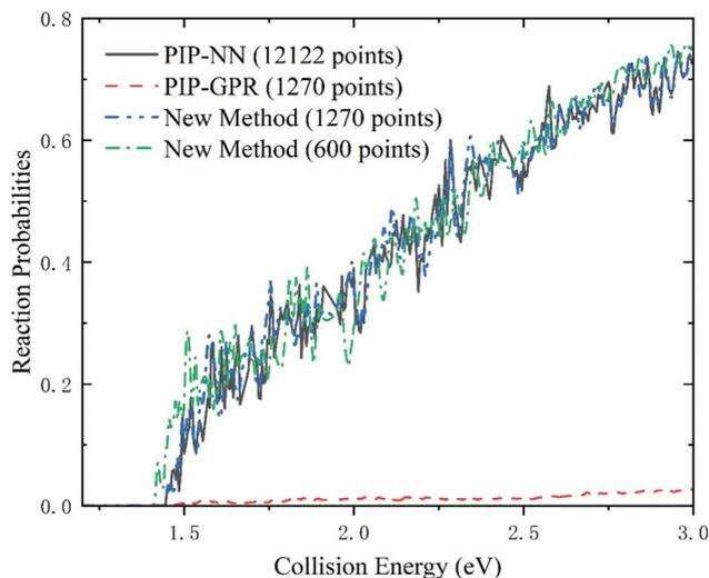
**Fig. 6** The total reaction probabilities of the Be<sup>+</sup>(<sup>2</sup>S) + H<sub>2</sub> → BeH<sup>+</sup> + H reaction with  $J = 0$  calculated on the PESs constructed by the PIP-NN model (12 122 points), the PIP-GPR model (1270 points), and the new method (600 and 1270 points).
