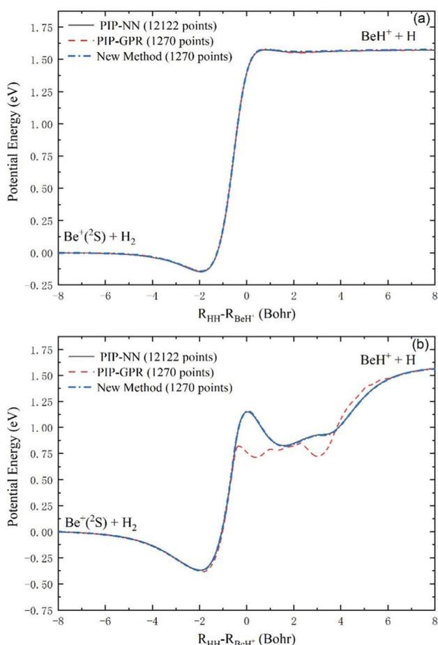
Fig. 5 Collinear (a) and global (b) minimum energy paths of the  $\text{Be}^+(\text{}^2\text{S}) + \text{H}_2 \rightarrow \text{BeH}^+ + \text{H}$  reaction calculated on the PESs constructed by the PIP-NN model (12 122 points), the PIP-GPR model (1270 points), and the new method (1270 points).
