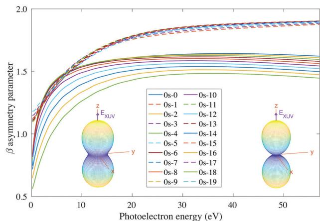
Fig. 9 Vibrationaly resolved  $\beta$  parameter for measurements in the ultracold regime ( $0s$  initial state) and ammonia's valence shell. Inset figures: corresponding photoelectron angular distributions for the  $\nu' = 16$  vibrational state of the cation at a photoelectron energy of 2 eV (left) and 50 eV (right).
