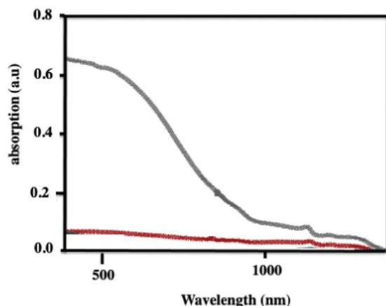
Fig. 6 Vis-NIR absorption spectra of  $\text{Fe}_3\text{O}_4$  nanocrystals either dispersed (black) or self-assembled to the produced supraballs (red). Reprinted with permission from ref. 34. Copyright 2020 John Wiley & Sons, Inc.
