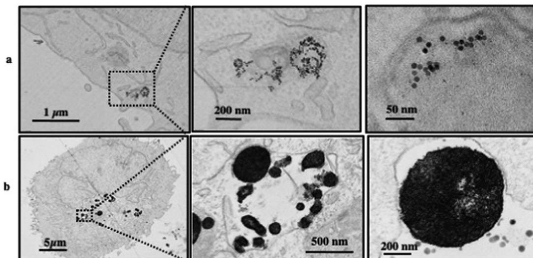
Fig. 8 2D TEM slice images at various enhancements of dispersed  $\text{Fe}_3\text{O}_4$  nanocrystals (a) and supraballs (b) in A431 tumor cells incubated for 1 day with  $28 \mu\text{g mL}^{-1}$  iron concentration.
