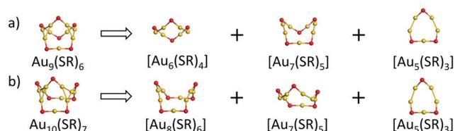
Fig. 2 Ring model-driven structural decomposition of (a) the  $[\text{Au}_9(\text{SR})_6]$  ring of  $\text{Au}_{21}(\text{SR})_{15}$  and (b)  $[\text{Au}_{10}(\text{SR})_7]$  ring of  $\text{Au}_{22}(\text{SR})_{16}$  into different rings. Au: yellow; S: red. The R groups are omitted for clarity.
