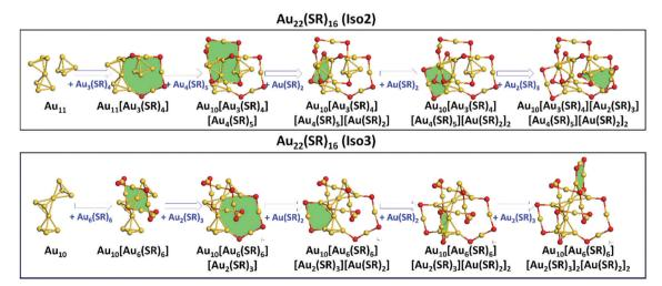
Fig. 4 The structural predictions of two Au<sub>22</sub>(SR)<sub>16</sub> isomers Iso2 (upper panel) and Iso3 (lower panel). Au: yellow; S: red. The rings were filled with green color. The R groups are omitted for clarity.
