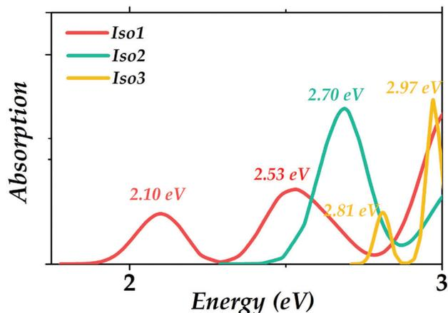
**Fig. 5** Calculated optical absorption spectra for the three Au<sub>22</sub>(SR)<sub>16</sub> (R = CH<sub>3</sub>) isomers.
