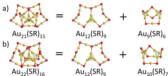
Fig. 1 Geometric decompositions of (a)  $\text{Au}_{21}(\text{SR})_{15}$  and (b)  $\text{Au}_{22}(\text{SR})_{16}$  ( $\text{R} = \text{SAdm}$ ). Au: yellow; S: red. The R groups are omitted for clarity.
