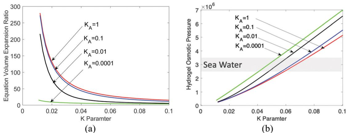
Fig. 11 (a) Equilibrium volume expansion ratio of polyelectrolyte hydrogel at a function of  $K$  parameter at different values of the equilibrium constant  $K_{PSA}$ , and (b) osmotic pressure of the hydrogel ( $\chi = 0$ ,  $\gamma = 2$ ).
