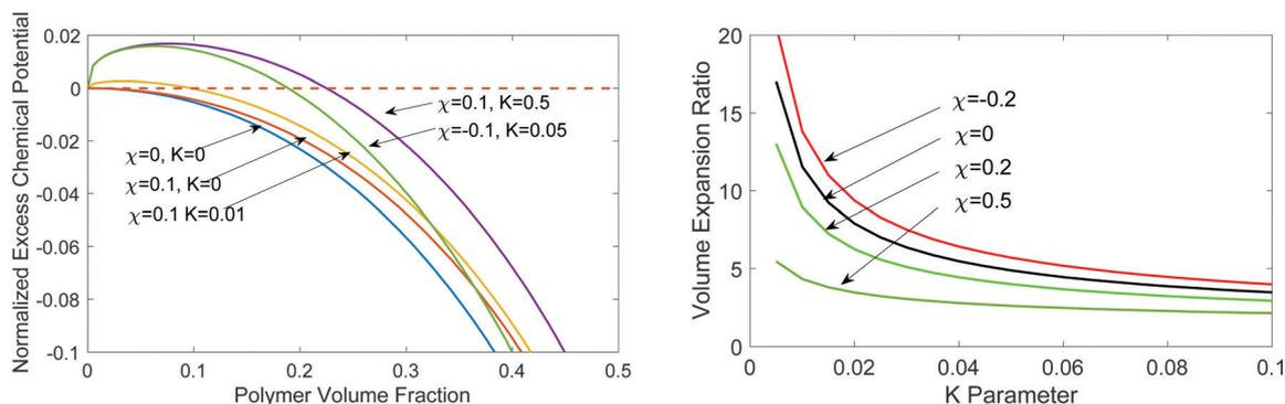
Fig. 1 (a) Normalized excess chemical potential of water  $[\mu_w(T, p) - \mu_w^o(T, p_o)]/(RT)$ , under different parameters, and (b) equilibrium volume expansion ratio as a function of parameter  $K$  under different  $\chi$  values.
