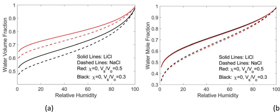
Fig. 7 Comparison of atmospheric water extraction, *i.e.* hydrogel water retention performance for hydrogel impregnated with LiCl and NaCl (a) water volume fraction and (b) water mole fraction as a function of humidity. The salt solubility in water set the lower limit of RH. Clearly, LiCl has better performance than NaCl due to its larger activity coefficients.
