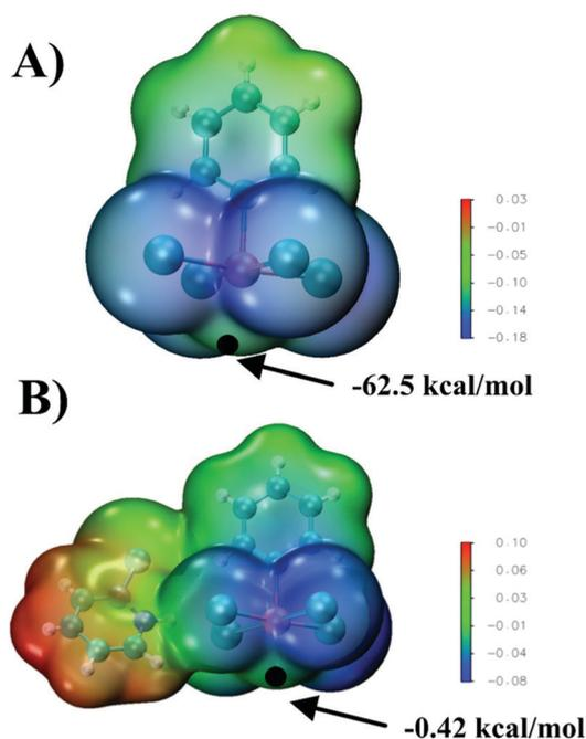
Fig. 2 MEP of the  $[\text{Te}(\text{C}_6\text{H}_5)\text{Cl}_4]^-$  monomer (A) and  $[\text{Te}(\text{C}_6\text{H}_5)\text{Cl}_4]^- \cdots \text{C}_5\text{H}_5\text{NBr}^+$  pair (B) on the 0.001 au isodensity surface. Black dot indicates  $V_{s,\text{max}}$  on the Te atom ( $\sigma$ -hole).
