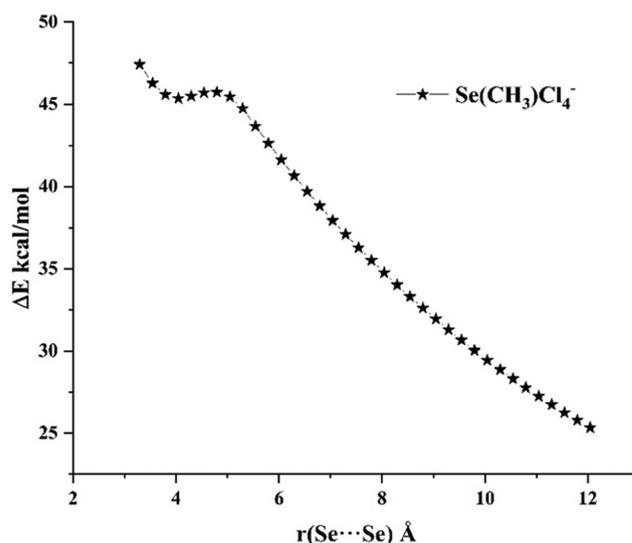
**Fig. 7** Dissociation profile of the Se(CH<sub>3</sub>)Cl<sub>4</sub><sup>-</sup> dimer in a vacuum.
