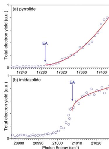
Fig. 6 Photodetachment spectra of (a) pyrrolide and (b) imidazolidine. The EA of each anion is indicated by the arrow. The photodetachment spectra are fitted by the Wigner threshold law:  $\sigma = A \times (h\nu - EA)^{l+1/2}$ , where  $A$  is the parameter related to the PE signal intensity,  $h\nu$  is the photon energy, and  $l$  is the angular momentum of the photoelectron. The  $l$  value is found to be 1.4 for (a) and  $-0.1$  for (b).
