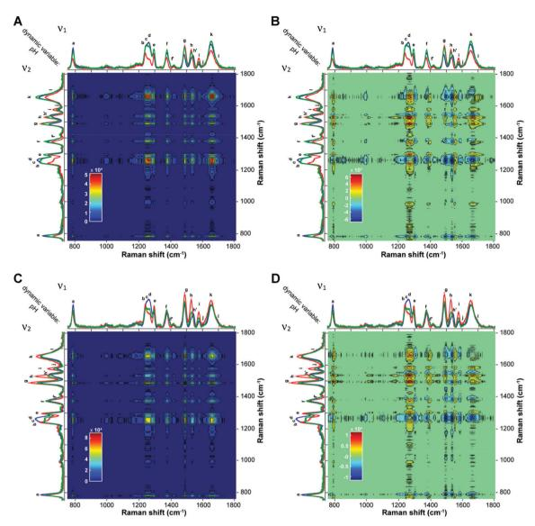
Fig. 6 Synchronous (A and C) and asynchronous (B and D) 2D UVRR correlation maps for *BCL2* (top) and *KRAS* (bottom) generated from the pH-dependent spectra. The color bar that applies to each map is displayed at the bottom left of the map.
