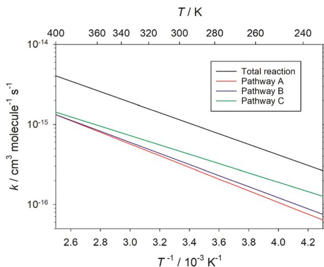
**Fig. 7** Arrhenius plot of the overall reaction between NO<sub>3</sub> and CH<sub>3</sub>BrI at a pressure of 1 bar N<sub>2</sub> and temperatures between 230 and 400 K, illustrating the overall reaction and the contribution from each of the pathways A, B and C.
