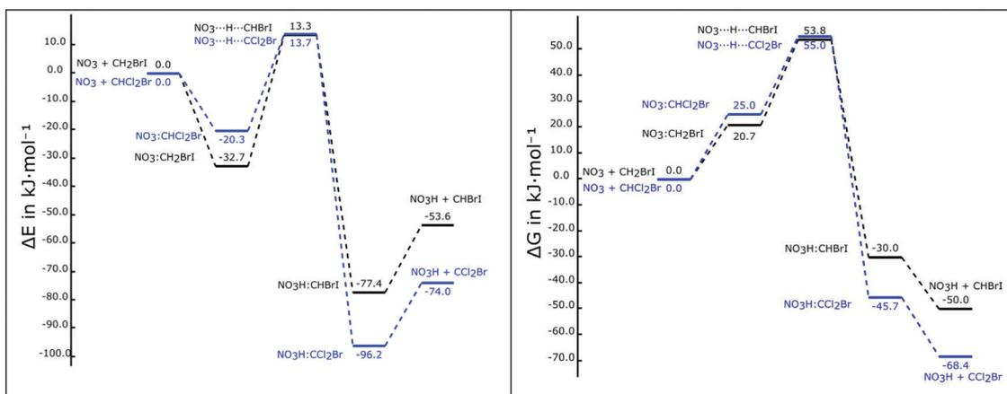
Fig. 5 Profiles of the relative electronic energy (left-hand panel) and Gibbs energy (right-hand panel) for the NO<sub>3</sub> + CH<sub>2</sub>BrI (black) and NO<sub>3</sub> + CHCl<sub>2</sub>Br (blue) reactions.
