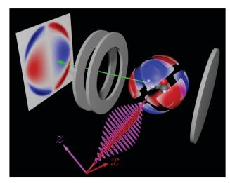
Fig. 4 Proposed velocity map imaging setup to measure the coefficient  $ilde{b}_{3,-2}$ :  $\omega$  (red wave) and  $2\omega$  (violet wave) are polarized along x and z, respectively. The detector projects the distribution on the x = z plane. Only the contribution of  $\tilde{b}_{3,-2}$  to the photoelectron angular distribution is shown. In red/blue regions there is an excess/deficit of photoelectrons.
