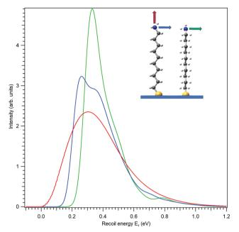
Fig. 4 Recoil lineshapes of the N 1s photoemission from a self-assembled monolayer (SAM) of aminodecanethiol molecules on surface. The emission direction is noted by the correspondingly coloured arrow in the inset (the molecule is slightly rotated around the vertical axis to make the shape more visible). Electron kinetic energy of 10 keV and the surface temperature of 20 K were used for the simulations.
