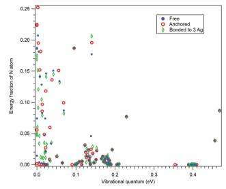
Fig. 3 The contributions of the N atom to the kinetic energy of all normal modes of 10-aminodecane-1-thiol, plotted against the energy of the vibrational quanta. The translational and rotational modes are at zero energy. Normal mode analysis was performed for three scenarios, as described in the text.
