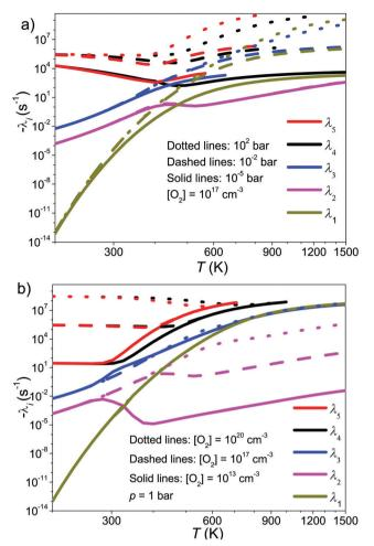
Fig. 7 Chemically significant eigenvalues of the CH<sub>2</sub>C(CH<sub>3</sub>)CH<sub>2</sub>• + O<sub>2</sub> reaction plotted as a function of temperature, pressure, and O2 concentration
