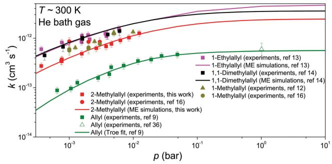
Fig. 6 Fall-off curves for allylic radical + O<sub>2</sub> reactions at around 300 K in helium bath gas.
