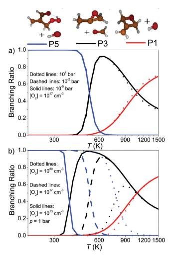
Fig. 8 Branching ratios of the products of the CH<sub>2</sub>C(CH<sub>3</sub>)CH<sub>2</sub>• + O<sub>2</sub> reaction plotted as a function of temperature, pressure, and O2 concentration.
