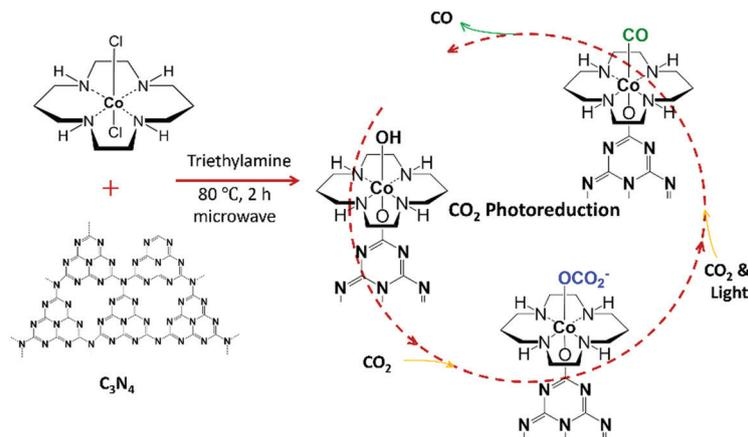
Fig. 1 Schematic representation showing the synthesis of Co-cyclam/C<sub>3</sub>N<sub>4</sub> and possible intermediates in photoreduction of CO<sub>2</sub> using the prepared catalyst in the presence of a sacrificial electron donor, triethanolamine (TEOA).
