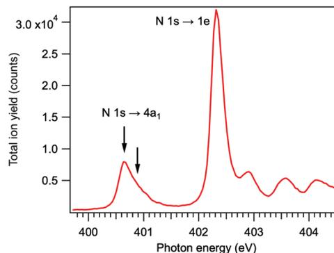
Fig. 2 Total ion yield spectrum of ammonia across the resonant excitations in the N 1s photoabsorption.
