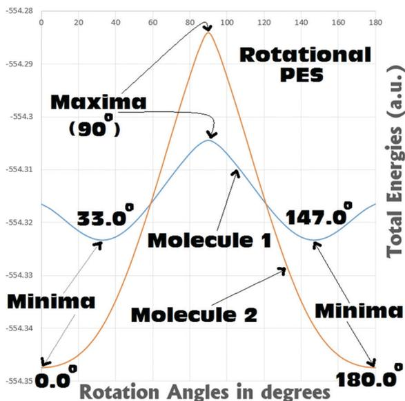
Fig. 5 Rotational potential energy surfaces (PES) of Molecules 1 and 2 computed using the  $\omega$ B97xD/6-31G(d,p) method. In this singlet PES, variation of rotational twist angles and energy only computations were carried out with the interval of  $5.0^\circ$ .
