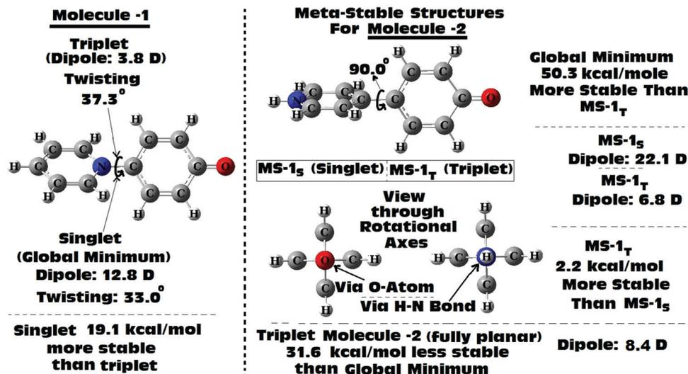
Fig. 6 Optimized structures of Molecules 1 and 2 computed using the  $\omega$ B97xD/6-31G(d,p) method, with some important data both in singlet as well as triplet surfaces shown. The energetics data shown are from the total energies of the stationary points.
