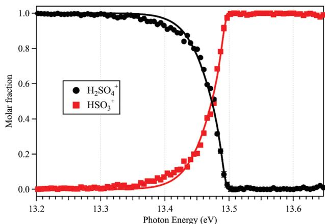
Fig. 4 Breakdown diagram of the  $\text{H}_2\text{SO}_4^+$  parent ion ( $m/z = 98$ ) and  $\text{HSO}_3^+$  fragment ion ( $m/z = 81$ ). Solid circles represent the experimental data, while lines correspond to the statistical model (see text for details).
