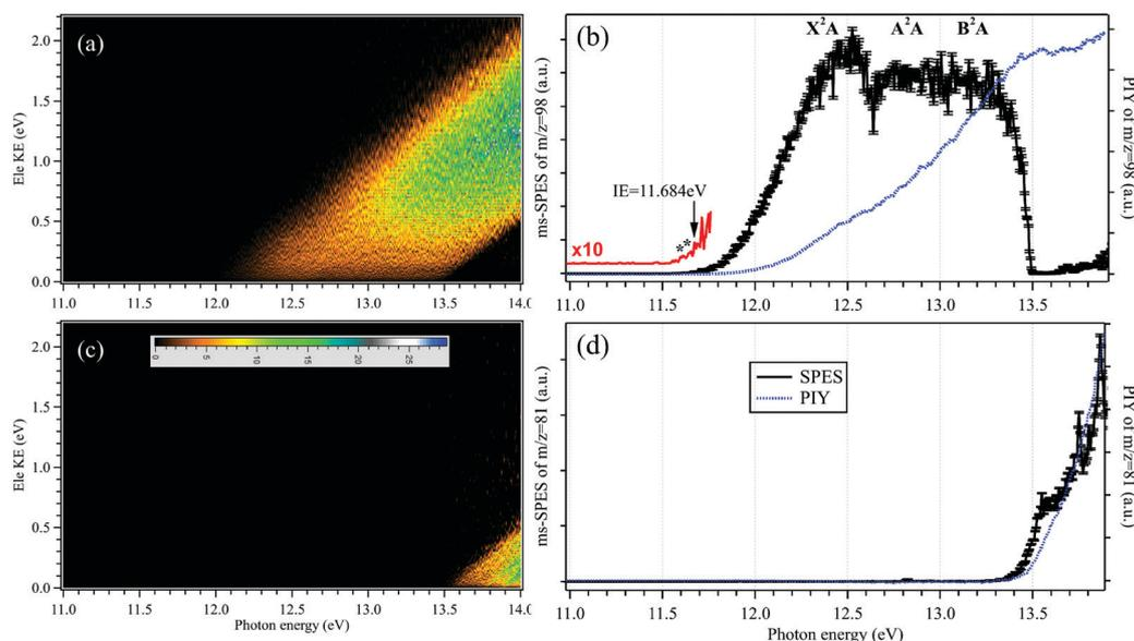
Fig. 2 Mass-selected photoelectron matrices, slow photoelectron spectra (SPES, black solid lines) and photoionization yields (PIYs, blue dotted lines) corresponding to (a and b) the  $\text{H}_2\text{SO}_4^+$  parent ion and (c and d) the  $\text{HSO}_3^+$  fragment ion. The 10 times magnified SPES in red shows the onset of  $\text{H}_2\text{SO}_4^+$ .
