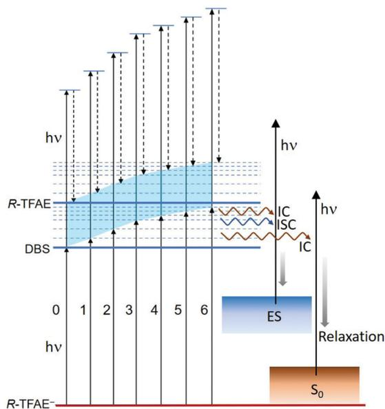
Fig. 7 Schematic energy level diagram showing the adiabatic detachment process from the bound vibrational levels of the DBS of  $R\text{-TFAE}^-$  by the second photon and the relaxation processes upon the first photon absorption. ES = excited states, IC = internal conversion, ISC = intersystem crossing.
