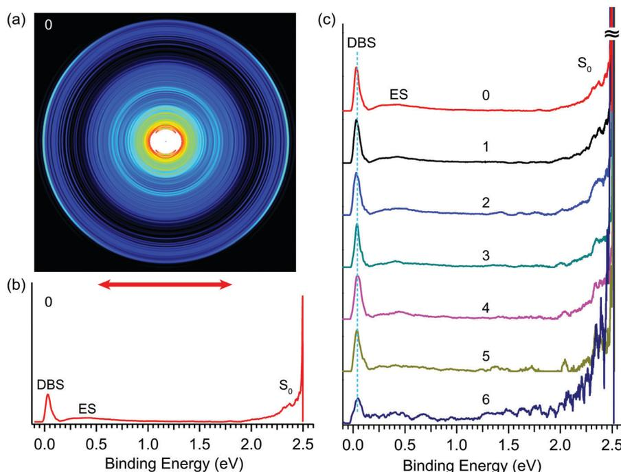
**Fig. 5** Resonant two-photon photoelectron images and spectra of  $R\text{-TFAE}^-$  at detachment wavelengths corresponding to peaks 0–6 shown in Fig. 4. (a) The photoelectron image at peak 0 (496.42 nm, 2.4975 eV); (b) the R2PD photoelectron spectrum inverted from the image in (a); the three observed features are labelled as DBS, ES, and  $S_0$ ; (c) comparison of the seven R2PD photoelectron spectra, the peak numbers from Fig. 4 are indicated, see Table 2 for the wavelengths of peaks 1–6.
