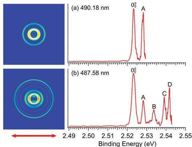
Fig. 3 Photoelectron images and spectra of *R*-TFAE<sup>−</sup> at (a) 490.18 nm (2.5294 eV) and (b) 487.58 nm (2.5428 eV). The double arrow below the images indicates the laser polarization.
