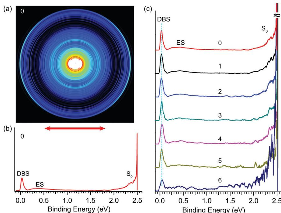
**Fig. 5** Resonant two-photon photoelectron images and spectra of  $R\text{-TFAE}^-$  at detachment wavelengths corresponding to peaks 0–6 shown in Fig. 4. (a) The photoelectron image at peak 0 (496.42 nm, 2.4975 eV); (b) the R2PD photoelectron spectrum inverted from the image in (a): the three observed features are labelled as DBS, ES, and  $S_0$ ; (c) comparison of the seven R2PD photoelectron spectra, the peak numbers from Fig. 4 are indicated, see Table 2 for the wavelengths of peaks 1–6.
