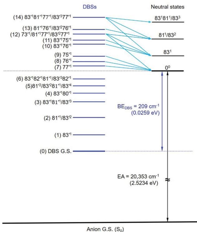
Fig. 8 The observed vibrational levels of the DBS of  $R\text{-TFAE}^-$  and the autodetachment processes from the vibrational Feshbach resonances to the neutral final states. The peak numbers in Fig. 4 are given in the parentheses.
