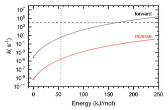
Fig. 4 Forward and reverse rate constants for crossing T5 between PA and **BCBdiene** (see Fig. 3 for reference). The dotted vertical line indicates the minimum energy present needed for the reaction to proceed. The horizontal line indicates the average residence time of molecules inside the pyrolysis microreactor.
