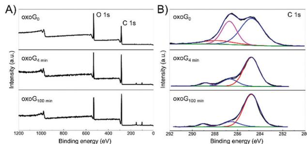
Fig. 3 (A) XPS survey spectra and (B) high-resolution C 1s XPS spectra of oxoG<sub>0</sub>, oxoG<sub>4 min</sub>, and oxoG<sub>100 min</sub> showing the changes of oxygen functional groups after sonication.
