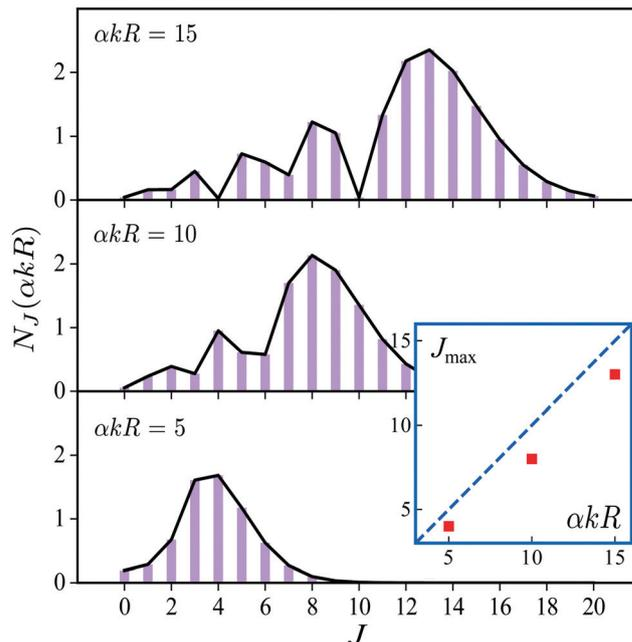
Fig. 2 Distribution  $N_J(\alpha_n R)$  (26) over  $J$  in the rotational recoil-induced wave packet (25) for different  $\alpha_n R$ . The red squares in the insert show the dependence of  $J_{\text{max}}$  on the recoil angular momentum  $\alpha_n R$ . Here  $J_{\text{max}}$  is the value of the angular momentum  $J$  when the distribution  $N_J(\alpha_n R)$  takes maximum. The dashed diagonal line in the insert corresponds to the recoil angular momentum  $J_{\text{rec}} = \alpha_n R$  (6).
