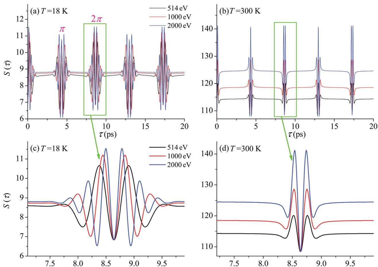
Fig. 4  $S(\tau)$  revival structure of the function (30) for the CO molecule computed at the low  $T = 18$  K (a and c) and room  $T = 300$  K (b and d) temperatures and for different energies of the photoelectron  $\varepsilon = 514, 1000$  and  $2000$  eV (see legends);  $\alpha_C = 0.571$ ,  $\theta = \angle(\mathbf{e}_1, \mathbf{e}_2) = 0$ .
