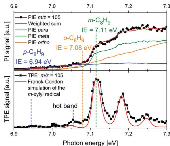
Fig. 8 In a *m*-xylene flame,  $m/z$  105 was identified, corresponding to xylyl radicals. The photoion signal (upper trace) does not permit identification of the product isomer. The TPE spectrum in the lower trace, on the other hand shows that *meta*-xylyl is the dominant product isomer and the band around 7.05 eV assigned to a hot band. The Figure was published in ref. 151, Copyright Elsevier, 2017.
