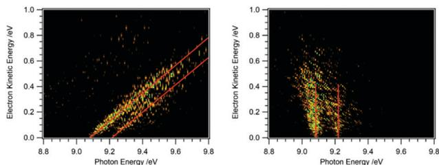
Fig. 2 2D map of the full photoelectron spectrum of HBBH with the vibrational bands indicated by the red diagonals (left-hand side).<sup>36,37</sup> A horizontal slice at 0 eV eKE corresponds to a TPE spectrum, a vertical slice at a given photon energy to the PES. After rotation of the matrix the 2D map on the right-hand side is obtained. Summing up horizontal slices yields a slow photoelectron spectrum, SPES, which often provides a better signal/noise ratio.
