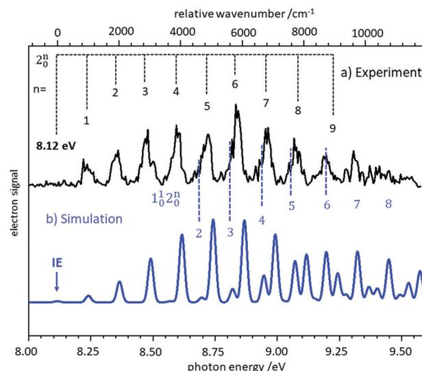
Fig. 3 Slow photoelectron spectrum of BH<sub>2</sub> (upper trace) compared with a Franck–Condon simulation. The IE was derived from the best agreement between experiment and simulation. Figure taken from ref. 61 by permission of the RSC.
