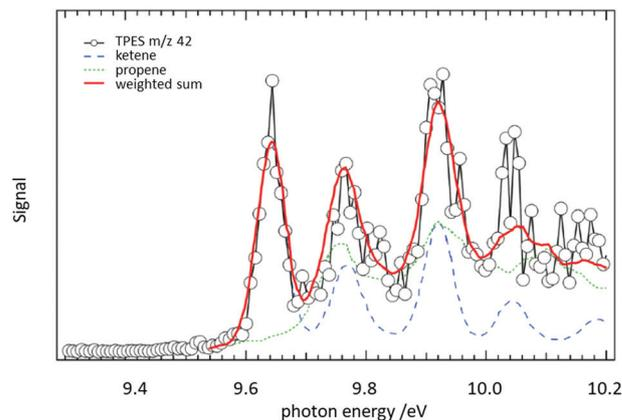
Fig. 9 The reaction of *n*-pentane with O<sub>2</sub> was studied in a jet-stirred reactor. From a fit to the ms-TPE spectra recorded at *m/z* 42, it was possible to extract a ketene/propene product branching ratio of 2 : 1. Reproduced from ref. 158 with permission from the Royal Society of Chemistry.
