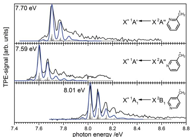
Fig. 7 Photoelectron spectroscopy allows the clear distinction of three isomers of the picolyl radical. (Figure taken from ref. 82 by permission of Wiley-VCH.)
