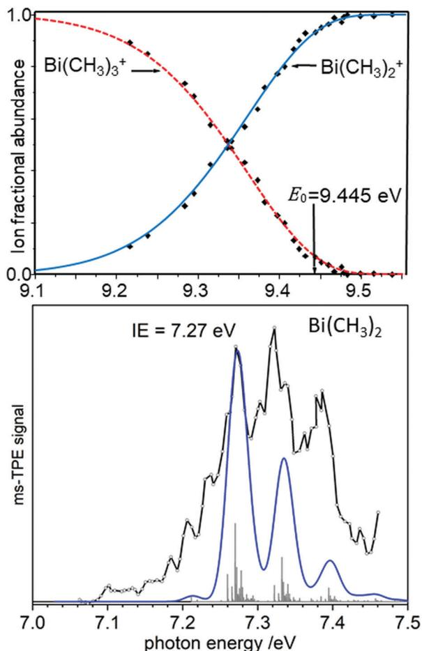
Fig. 6 The appearance energy  $AE_{0K}(\text{Bi}(\text{CH}_3)_3, \text{Bi}(\text{CH}_3)_2^+)$  has been determined from a breakdown diagram (upper trace, here labelled  $E_0$ ). Combined with the IE of  $\text{Bi}(\text{CH}_3)_2$  (lower trace) a Bi-CH<sub>3</sub> bond dissociation energy is obtained. Upper trace: Redrawn with permission from ref. 120, Copyright 2009, American Chemical Society. Lower trace: Reproduced from ref. 121 with permission of the Royal Society of Chemistry.
