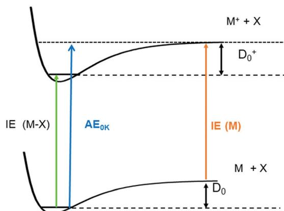
Fig. 4 Dissociation energies,  $D_0$ , can be determined by combining the appearance energy  $AE_{0K}(MX, M^+)$  of a molecule with the ionisation energy of the radical  $M$ ,  $IE(M)$ . Combination of the AE with the IE of the molecule  $IE(MX)$  yields  $D_0^+$  in the ion.
