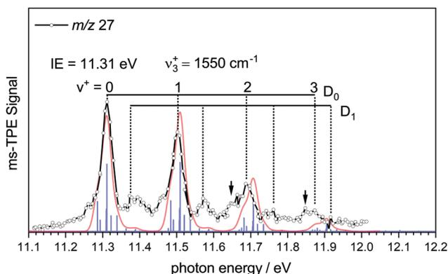
Fig. 2 ms-TPES of HBNH with a harmonic simulation based on the computed geometry, performed at 1100 K (red line). The IE was determined to be  $11.31 \pm 0.02$  eV and a progression of  $1550 \text{ cm}^{-1}$  in the BN stretching mode of the cation was observed.
