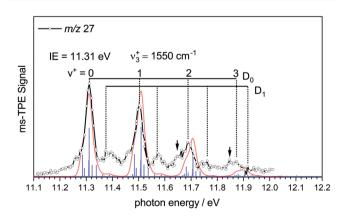
Fig. 2 ms-TPES of HBNH with a harmonic simulation based on the computed geometry, performed at 1100 K (red line). The IE was determined to be 11.31  $\pm$  0.02 eV and a progression of 1550 cm $^{-1}$  in the BN stretching mode of the cation was observed.
