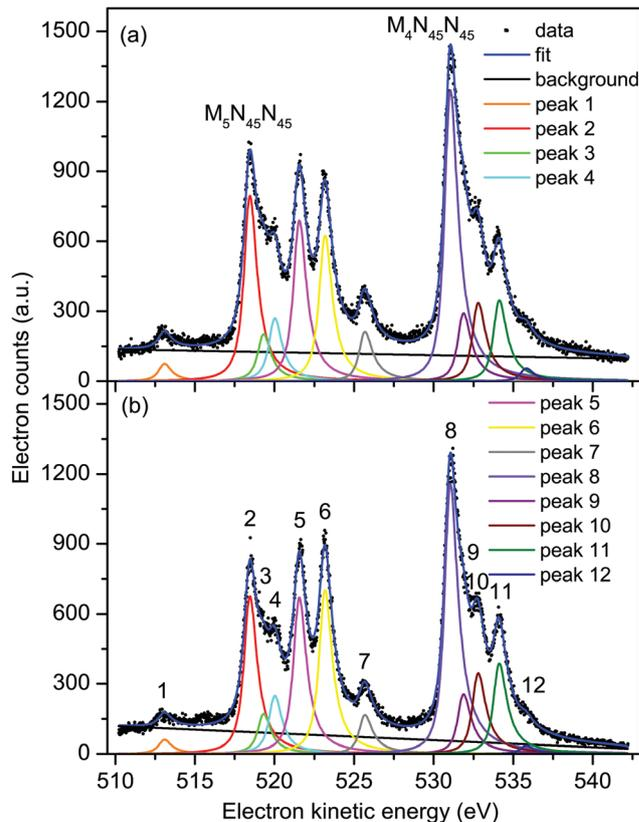
Fig. 3 Non-resonant Auger electron bands due to the  $M_{45}N_{45}N_{45}$  transitions in  $XeF_2$  recorded with parallel (a) and perpendicularly (b) polarized radiation at a photon energy of 710 eV. The raw and the fitted data are shown (see text for details). The kinetic energies of the peaks numbered 1–12 are given in Table 1.
