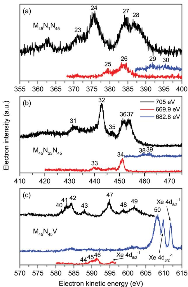
**Fig. 4** The non-resonant ( $h\nu = 705$  eV), and resonantly excited ( $h\nu = 669.9$  and  $682.8$  eV) Auger electron spectra of  $XeF_2$  showing bands due to the Xe  $M_{45}N_1N_{45}$  (a), Xe  $M_{45}N_{23}N_{45}$  (b) and Xe  $M_{45}N_{45}V$  and F KVV (c) transitions. All of these spectra were measured with perpendicularly polarized radiation. The kinetic energies of the peaks numbered 23–50 are given in Table 3.
