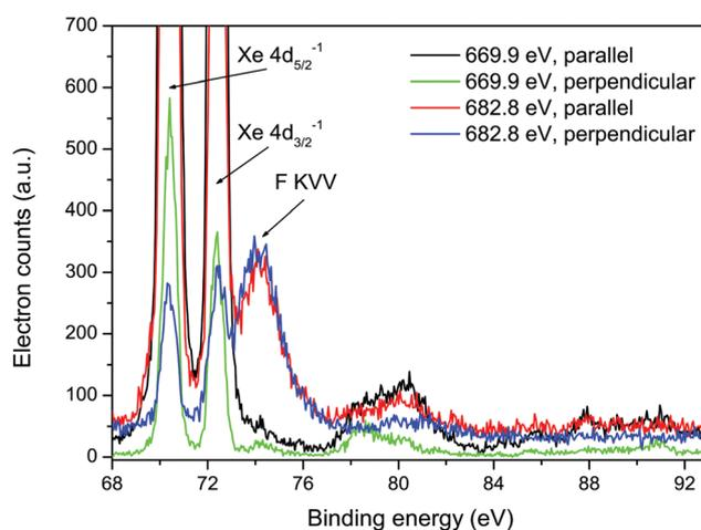
**Fig. 5** Resonantly excited electron spectra recorded at photon energies of 669.9 and 682.8 eV, using parallel and perpendicularly polarized radiation, plotted as a function of binding energy. The two intense peaks at binding energies of 70.38 and 72.39 eV arise from the Xe  $4d_{5/2}^{-1}$  and  $4d_{3/2}^{-1}$  states, and the structure observed between  $\sim 77$  and 83 eV is due to the associated shake-up satellites.<sup>6</sup>
