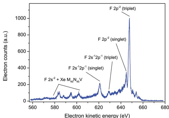
Fig. 6 The fluorine KVV and xenon M<sub>45</sub>N<sub>45</sub>V Auger electron spectrum in XeF<sub>2</sub>, recorded at a photon energy of 800 eV, using perpendicularly polarized radiation. The peaks have been labelled as F 2p<sup>-2</sup>, 2s<sup>-1</sup>2p<sup>-1</sup> and 2s<sup>-2</sup> (triplet or singlet) in a manner analogous to those predicted for SiF<sub>4</sub>.<sup>5</sup>
