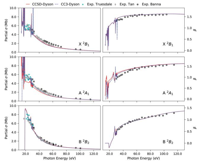
Fig. 2  $H_2O$ . Partial cross-section  $\sigma$  (left panels) and asymmetry parameter  $\beta$  (right panels) for the primary ionization channels obtained using EOM-CCSD and EOM-CC3 Dyson orbital descriptions of the bound state. B-spline TD-DFT is used for the continuum orbital description. Experimental results are taken from ref. 90-92.
