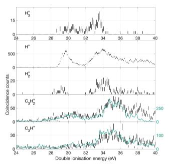
Fig. 10 Double ionization spectra based on two electrons detected in coincidence with a singly charged ion as specified for each spectrum. Both two-body and three-body fragmentation can contribute to these spectra, but two-body decays are probably dominant. The green line in the two lowermost panels are the number of counts found when correcting for a large peak overlap in m/q = 36-40.
