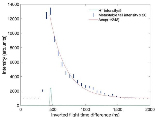
**Fig. 8** Metastable tail intensity as a function of the inverted flight time difference with a fit to the exponential decay in red. The coincidences are the same as in the tail in Fig. 7 plotted against  $t_2 - t_1$  where  $t_1$  and  $t_2$  are the flight times of the first and second ion to be detected, respectively. The location of the mass peak for  $\text{H}^+$  ions on the same scale is included below the decay curve for comparison.
