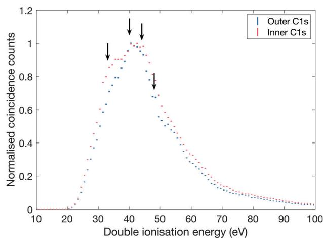
**Fig. 3** Double ionization spectra of allene measured with 300.5 eV photon energy. The spectra have been selected on outer and inner C1s core electron, respectively. The inner C1s electron has a binding energy of 290.8 eV and the outer C1s electron has 290.6 eV,<sup>29</sup> and the selections comprise binding energy ranges of  $\pm 0.1$  eV. The arrows indicate structures in the ionization spectra at energies of about 33, 40, 44 and 48 eV.
