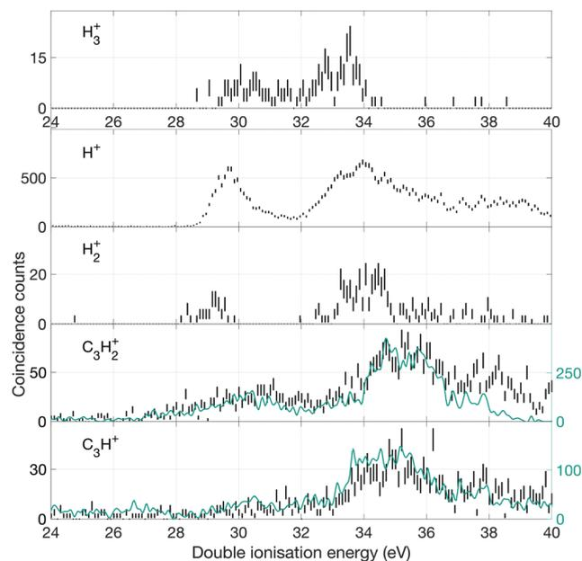
**Fig. 10** Double ionization spectra based on two electrons detected in coincidence with a singly charged ion as specified for each spectrum. Both two-body and three-body fragmentation can contribute to these spectra, but two-body decays are probably dominant. The green line in the two lowermost panels are the number of counts found when correcting for a large peak overlap in  $m/q = 36-40$ .
