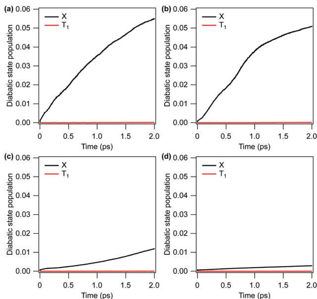
Fig. 3  $\tilde{X}$  and  $\tilde{T}_1$  diatomic state populations within 2 ps calculated following the selective population of the out-of-plane bending ( $Q_4$ ) and C–O stretching ( $Q_2$ ) modes in the  $\tilde{A}$  state. (a)  $Q_2^4 Q_4^1$  (304 nm), (b)  $Q_2^3 Q_4^1$  (314 nm), (c)  $Q_2^2 Q_4^1$  (329 nm), (d)  $Q_2^1 Q_4^1$  (337 nm).
