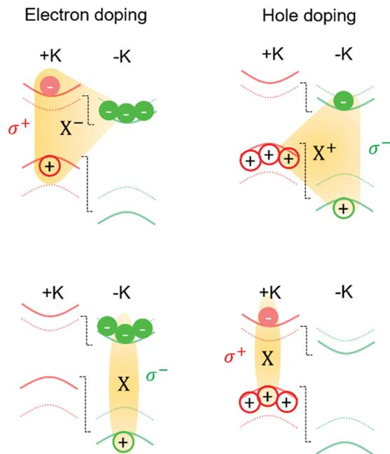
Fig. 3 Schematics of valley selective exciton-charge dressing in 1L MoSe<sub>2</sub> in an external magnetic field. Only the lowest conduction and highest valence bands are shown. Dotted curves: 0 field; solid curves: 9 Tesla. Due to Zeeman shift, electrons and holes preferentially populate  $-K$  and  $+K$  valleys, and dress excitons in  $+K$  and  $-K$  valleys, respectively.
