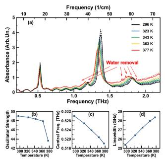
Fig. 2 (a) Evolution of the THz absorption spectrum with temperature, solid lines – retrieved in the experiment, dashed lines – fit results. (b-d)Evolution of, respectively, the strength, central frequency and linewidth of an oscillator used to fit the experimental time-trace and corresponding characteristic α-lactose monohydrate absorption line at ~0.53 THz.
