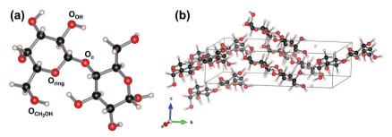
Fig. 5 Ball-and-stick representation of a gas-phase molecule  $\alpha$ -lactose (a) and the hygroscopic  $\alpha$ -lactose molecular crystal (b). The unit cell of the latter is indicated with a box. The different O sites are indicated in the gas-phase molecule.
