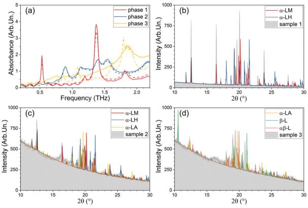
(a) THz absorbance spectra of the three phases at the room temperature: solid lines – the ones discussed in Sections 3.1.–3.3. (pellets heated in the mount with integrated heating), dashed lines - the ones of the pellets prepared for the XRD experiment (heated in the TGA setup). (b-d) XRD data: grey curves – obtained for the studied samples (1–3, correspondingly), colour lines – simulated results for the corresponding lactose crystallographic phases
