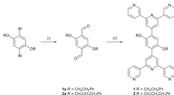
Scheme 4 Synthetic route to **1** and **2**. Reagents conditions (see ESI† for full details): (i) *n*-BuLi, Et<sub>2</sub>O, 0 °C; dry DMF, warmed to room temperature, 22 h; (ii) 3-acetylpyridine, KOH, NH<sub>3</sub>, EtOH, RT, 6 days for **1** and 5 days for **2**.
