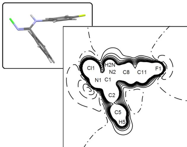
**Fig. 6** Electrostatic potential map of NCLBA extracted from the crystal in the Cl1–N1–C1 plane, as evaluated from periodic quantum simulation of the experimental structure ( $T = 17.5$  K) at the PBE0 level of theory, in conjunction with the Peintinger’s basis set. Contour levels are in atomic units, at steps of 0.02 au. Full lines: positive contours. Dashed: negative. Point-dashed: zero level. The inset shows the molecular orientation of the map.
