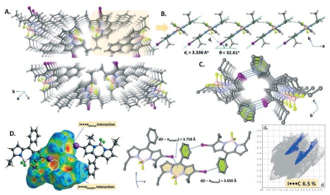
Fig. 3 (A) Perspective view of the crystal packing of B1. (B) Illustration of the 1D domino-like arrangement running along the a-axis. (C) Perspective view of the tubular-like architecture in the crystal packing of **B1** through the  $I \cdots \pi_{phenyl}$  interactions. (D) Hirshfeld surface of **B1** mapped with  $d_{\text{norm}}$  and the 2D fingerprint plot representing the I $\cdots$  $\pi_{\text{phenyl}}$  and I $\cdots$  $\pi_{\text{BODIPY}}$  interactions.
