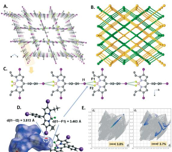
Fig. 7 (A) View of the 3D halogen-bonded framework showing a single network in the crystal packing in **B5**. (B) Illustration of two-fold halogen-bonded interpenetration formed through  $-BF_2\cdots I$  and  $I\cdots I$  contacts. (C) View of the directional symmetrical bifurcated  $-BF_2\cdots I$  XB contacts forming a 1D chain in **B5**. (D) and (E) Hirshfeld surface representations of symmetrical bifurcated  $-BF_2\cdots I$  and  $I\cdots I$  XBs showing the 2D fingerprint plots.
