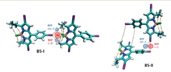
Fig. 13 Molecular graph of the B5 dimers.
