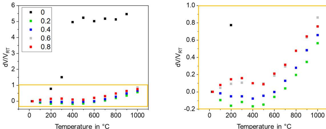
Fig. 7 Thermal expansion of Ba<sub>1-x</sub>Sr<sub>x</sub>Zn<sub>2</sub>Si<sub>2</sub>O<sub>7</sub> as a function of the temperature for various *x*-values.
