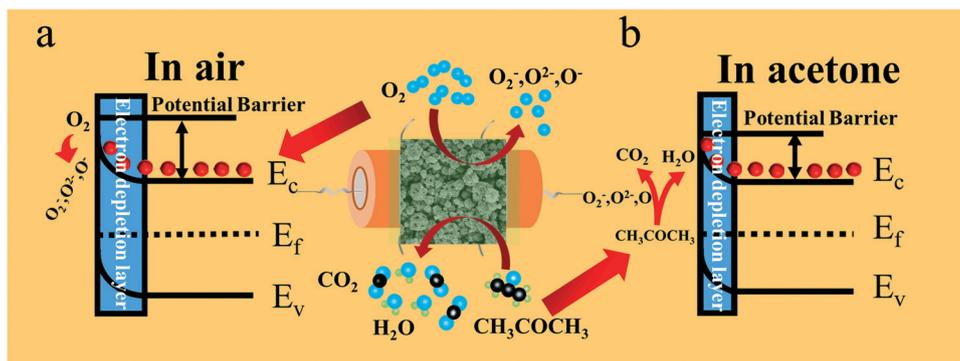
Fig. 8 Schematic illustration of the depletion theory and the sensing mechanism of the ZnO samples in air (a) and acetone vapor (b).
