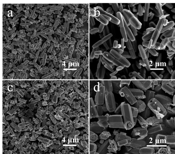
Fig. 3 FESEM images of (a and b) ZnO-DR and (c and d) ZnO-HR.
